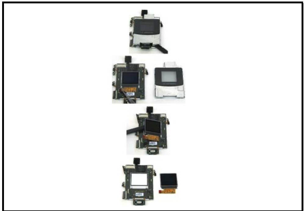
Figure 16. Removing the Display Module Lens
