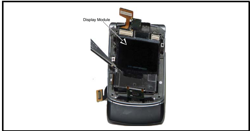
Figure 15. Removing the Display Module Assembly
