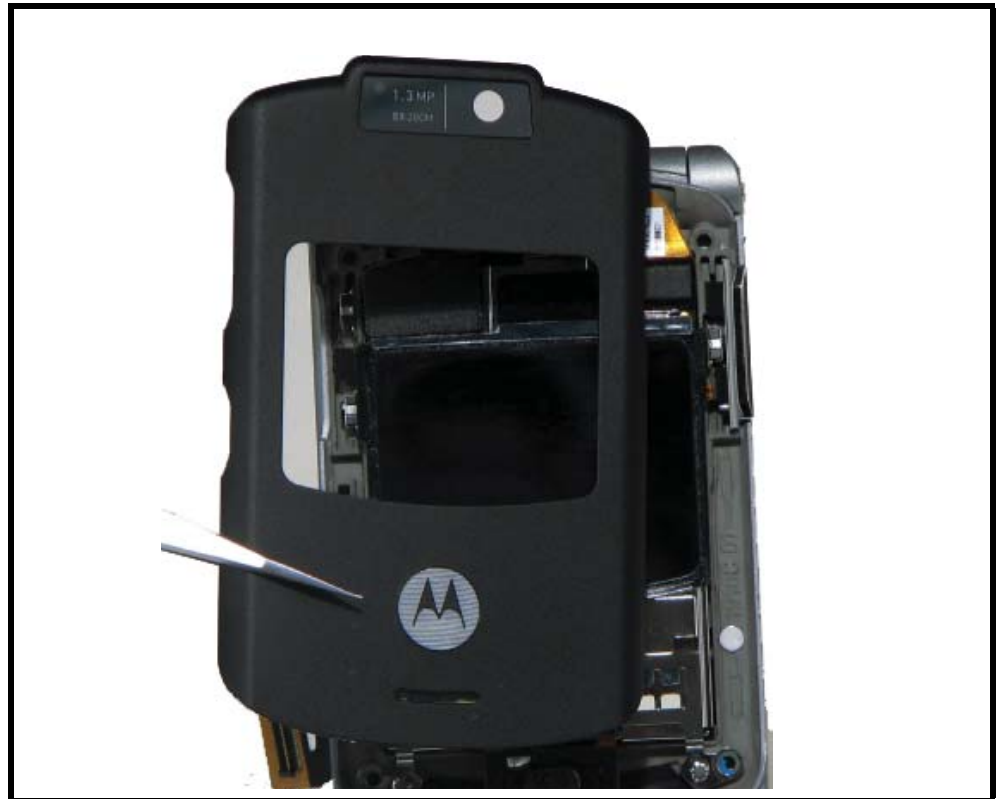
Figure 12. Removing the Flip Assembly Cover
