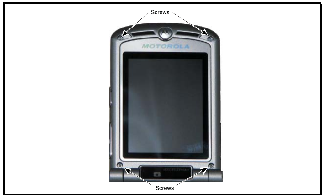
Figure 10. Removing the Flip Assembly Screws
