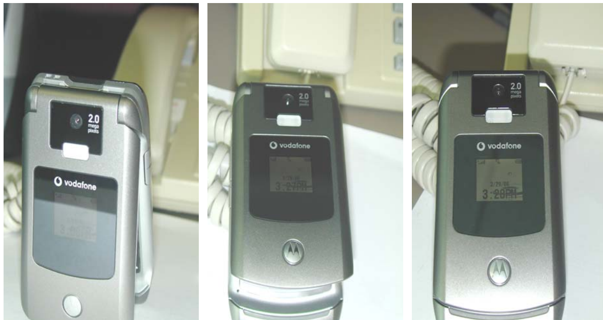
CLI on with flip open at 35° CLI on, ~ 10° before closing
