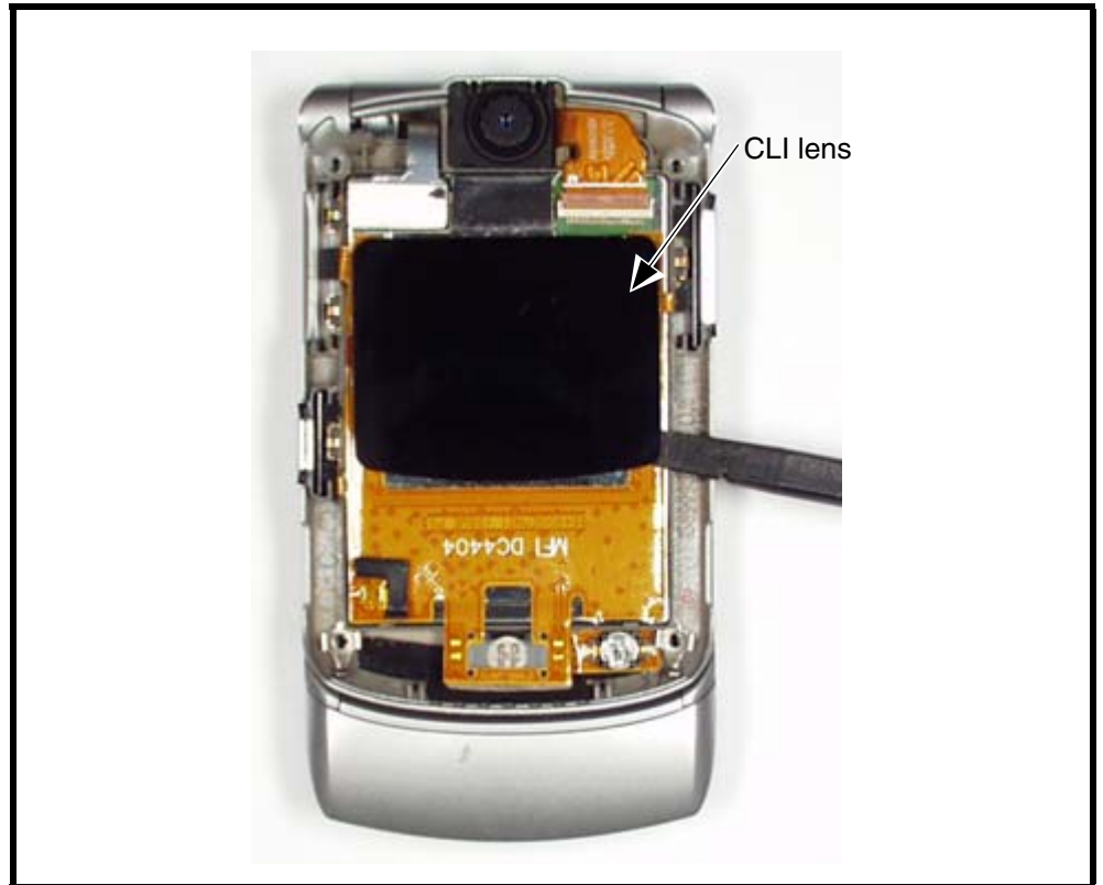
Figure 16. CLI Lens Removal
