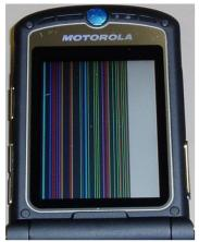
The cause of the crack driver IC was determined to be physical force being applied at the Main lens by the Motorola Logo. Sharp displays are more susceptible to this issue due to its mechanical characteristics.
