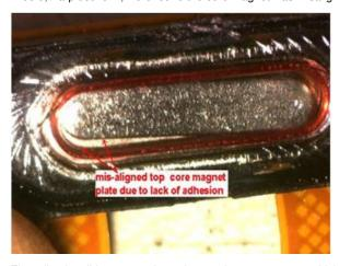
The adhesive did not spread evenly over the core magnet, which caused the core magnet to shift and generate low or distorted sound. The poor distribution of adhesive was due to the uneven pressure imposed on the core magnet.
