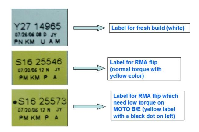
Note: The flip assembly label is only visible after disassembly of the rear housing.
