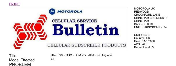
Service is aware that some GSM V3i phones from Brasil have been returned with customer complaints related to Alert – No Ring The failure mode analysis revealed that the inductor L1422, Part Number 2471992B42 is being damaged in the manufacturing ar assembly process, thus causing customer to notice a difficult with ringtones - no alert audio. See pictures below :
