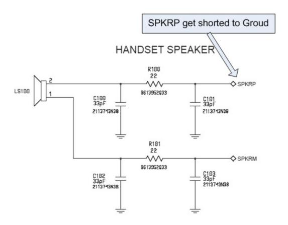
There are two main contributing factors, the placement of the kapton tape and the burr on the display bezel. First the kapton intended to protect the P-Flex from the display bezel edge which has burr was not being placed correctly during the assembl thus allowing the bezel burr to come into contact with the flex. Second the burr created during the stamping of the display be found to be sharper that expected, which allows the burr to become more dangerous to the P-Flex.
