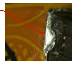
The Cross-Section confirmed that the speaker pad has been disconnected at copper level. See the pictures shown below.
