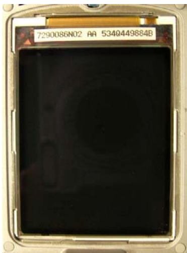
7290086N02 Note the label on display driver Supplier: Sharp
