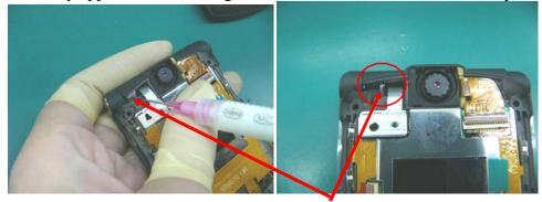
3. Open and close flip twice to ensure the lubricant is spread.
