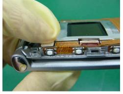
2. Evenly applied 1mm (5~8mg) of the lubricant into the end of endcap shaft.
