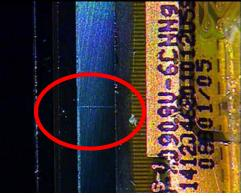
The cause of the crack driver IC was determined to be physical force being applied at the CLI lens.
