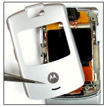
4. Heat up the CLI Lens with a Temperature of 100°C (212° F) for 20 sec and slide carefully in use of the flat end of the plastic tool, between Lens and metal frame.
