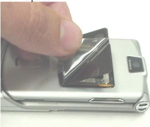
The root cause was determined to be the display chassis getting deformed when removing the old CLI lens from the phone at the service center. This causes a plate spring effect which may lift up the CLI lens after some time after rework.
