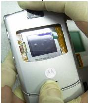
2. Align the outer and inner flip at left side; press right and top hooks.
