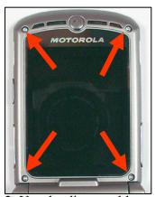
2. Use the disassembly tool to release cover latches on each side of the Front cover.
