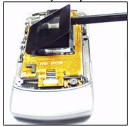
8. Carefully remove the rest of glue in use of the plastic tool. Do not use any kind of liquid or spray!
