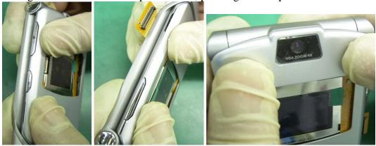
3. Place the pre-assembly CLI lens, apply pressure at the corners and hold the lens down for 5 sec to ensure good adhesion.
