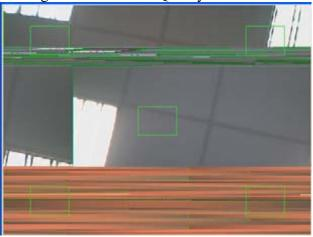
The root cause was determined to be soldering joint issue on the camera module cause by insufficient solder paste.
