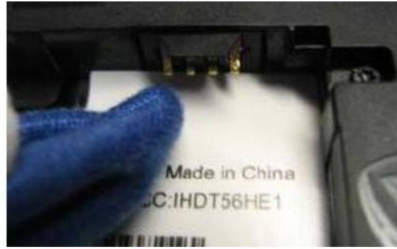
Figure 5 - Cleaning Battery Contacts with Lint Free Cloth and IPA
