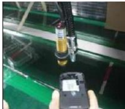
Figure 7 - Cleaning Battery Contacts with Ionized Air
