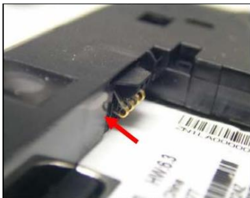
MEZNT46001A Battery block (old) pins curling up (see arrow)
