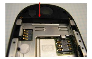
Long-Term: The M1400 battery contacts have been redesigned to eliminate this failure mode. The new part number 3987697Y05 replaces the old part number 3987697Y02 for reference designator M1400. See Images Below.
