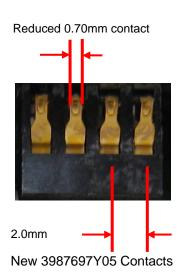
Factory cross-over the new part number was completed December 1<sup>st</sup>, 2005 and coordinated with an up-suffix of the PCBA and XCVR model numbers from AA to BA. PCBA and XCVR Model Numbers ending in AA have the old part number 3987697Y02. PCBA and XCVR Model Numbers ending in BA or CA have the new part number 3987697Y05.
