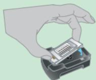
2. Charging the battery pack with a desk charger (use after connecting to a travel charger)
