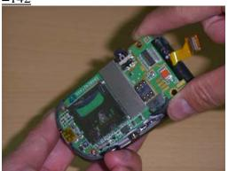
3. Remove the shield which has the EL module glued. Be careful not to damage PCB components. Remove the glued EL module from the shield and clean the glue residues from the shield.
