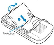
Inserting/Removing the Battery Pack
