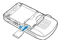
Insert the microSD memory card correctly. If the card is not inserted correctly, the card cannot be used.
