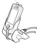
When connecting the USB cable (bundled accessory), connect it to the FOMA handset before attaching
