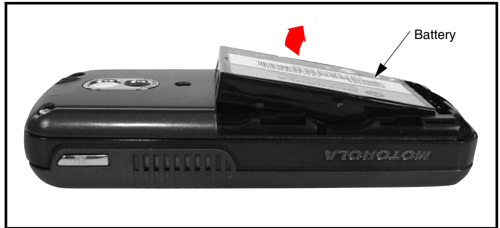
Figure 5. Removing and Replacing the Battery
