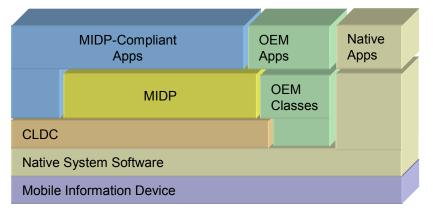
The Configuration Layer used in the E380 is the Connected Limited Device Configuration 1.0 (CLDC 1.0) and the Profile Layer used is the Mobile Information Device Profile 1.0 (MIDP 1.0). Together, the CLDC and MIDP provide common APIs for I/O, simple math functionality, UI, and more.
