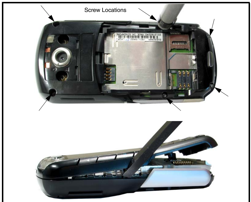
Figure 6. Removing the Front Housing
