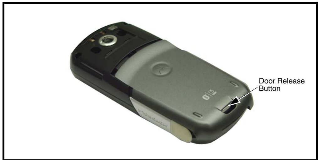
Figure 3. Removing and Replacing the Battery Door
