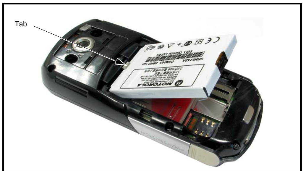
Figure 4. Removing and Replacing the Battery
