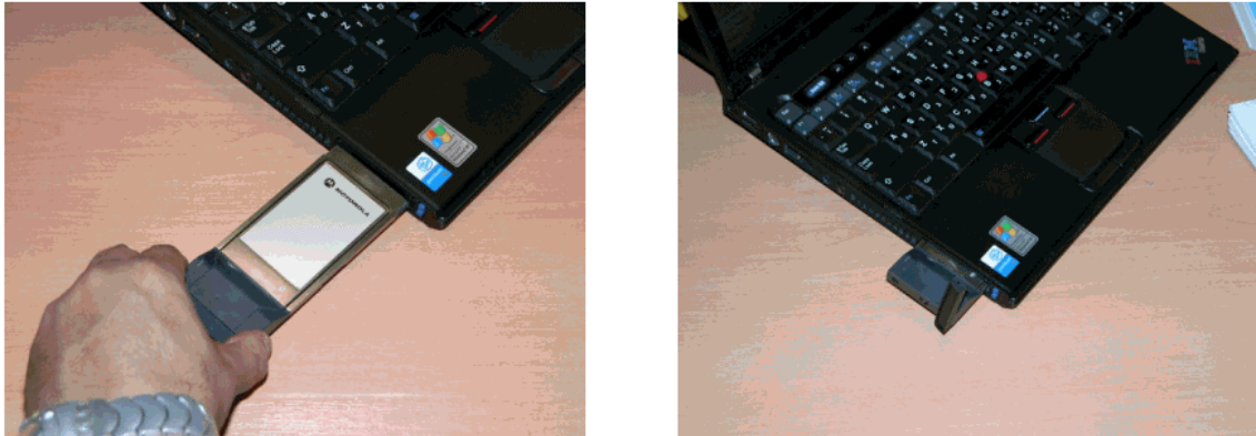
Figure 5. Mounting the D1000 Card
