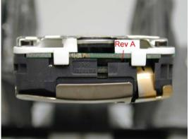
2) Disassemble the endo assy from the PCB. Inspect U902. Replace if damaged or missing
