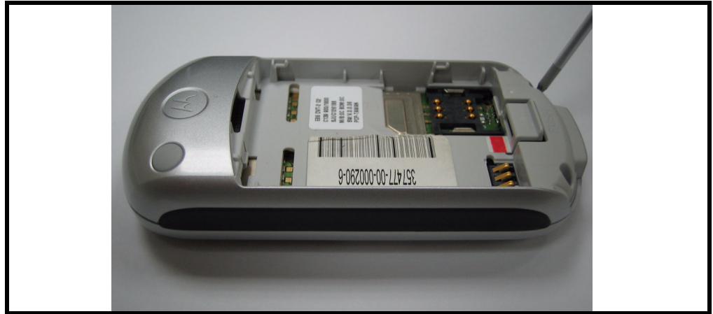
Figure 9. Removing the two T5 screws (T-force = 1.4 kgf-cm)
