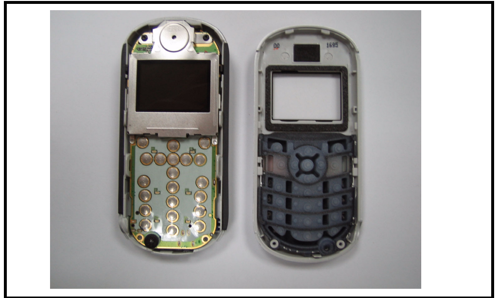
Figure 11. Removing the front housing
