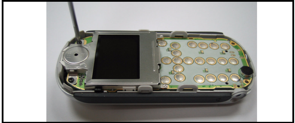
Figure 13. Removing two T5 screws (T-force = 1.4 kgf-cm)
