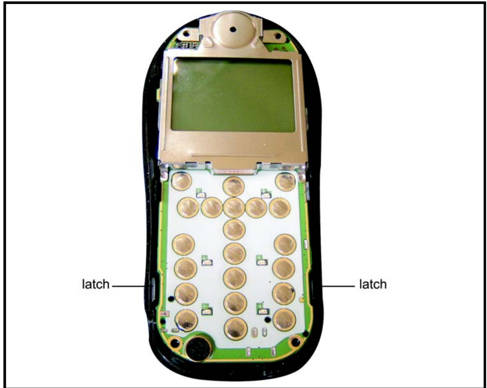
Figure 12. Pry open the side latches securing the Transceiver board to the back housing
