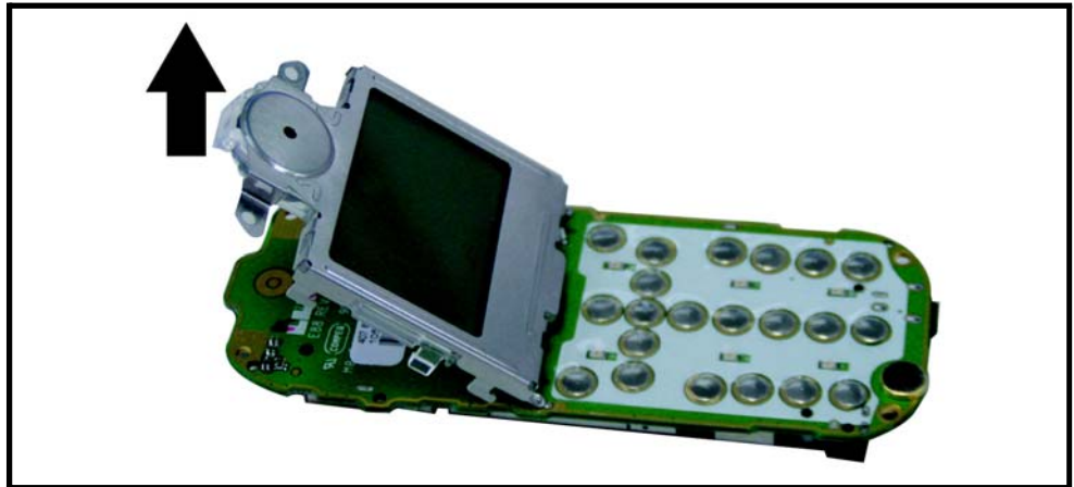
Figure 15. Pry the LCD screen away from the Transceiver board
