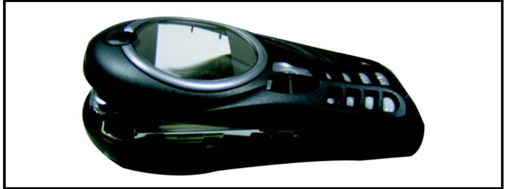
Figure 9. Remove the front housing
