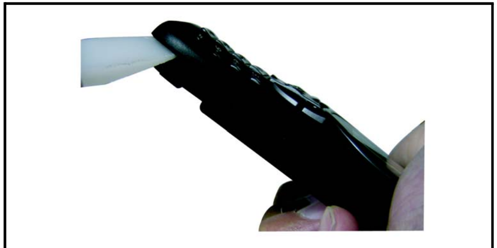
Figure 8. Use a flat wedge tool to pry the case
