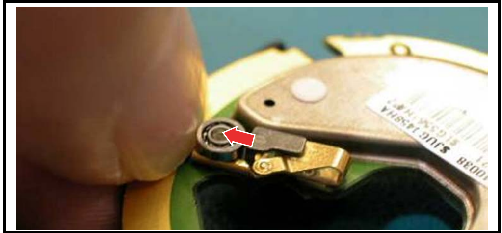
Figure 76. Pushing the Detent Bearing-Slider Assembly
