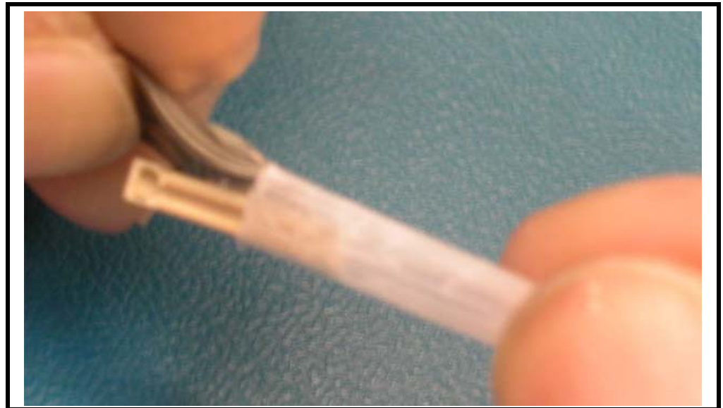
Figure 21. Protecting the Coaxial Connector Protective Cap
