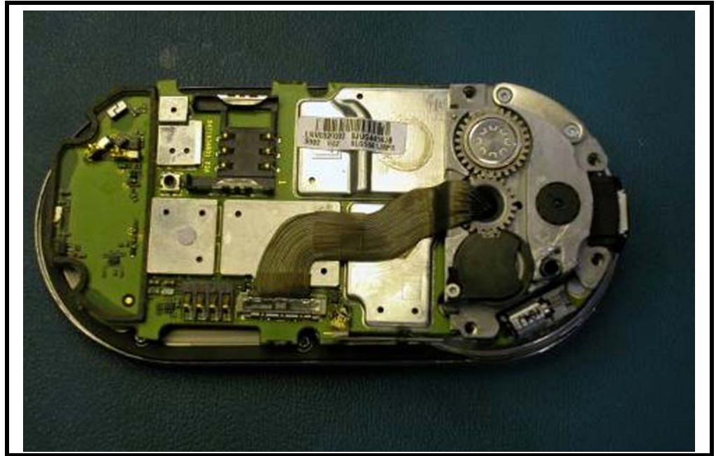
Figure 97. Inspecting the Coax Assembly
