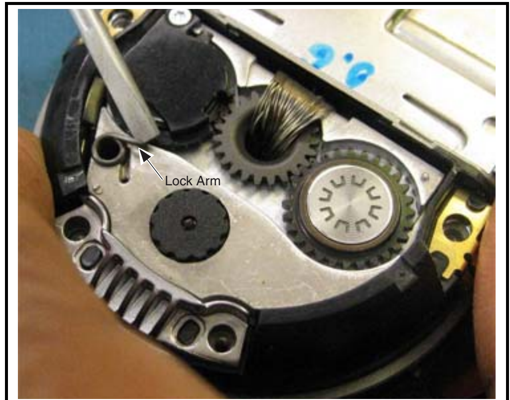
Figure 104. Setting the Detent Torsion Spring
