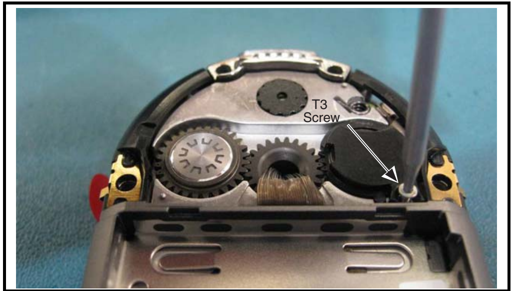
Figure 15. Securing the Timing Lock
