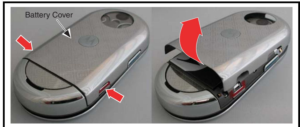
Figure 4. Removing the Battery Cover
