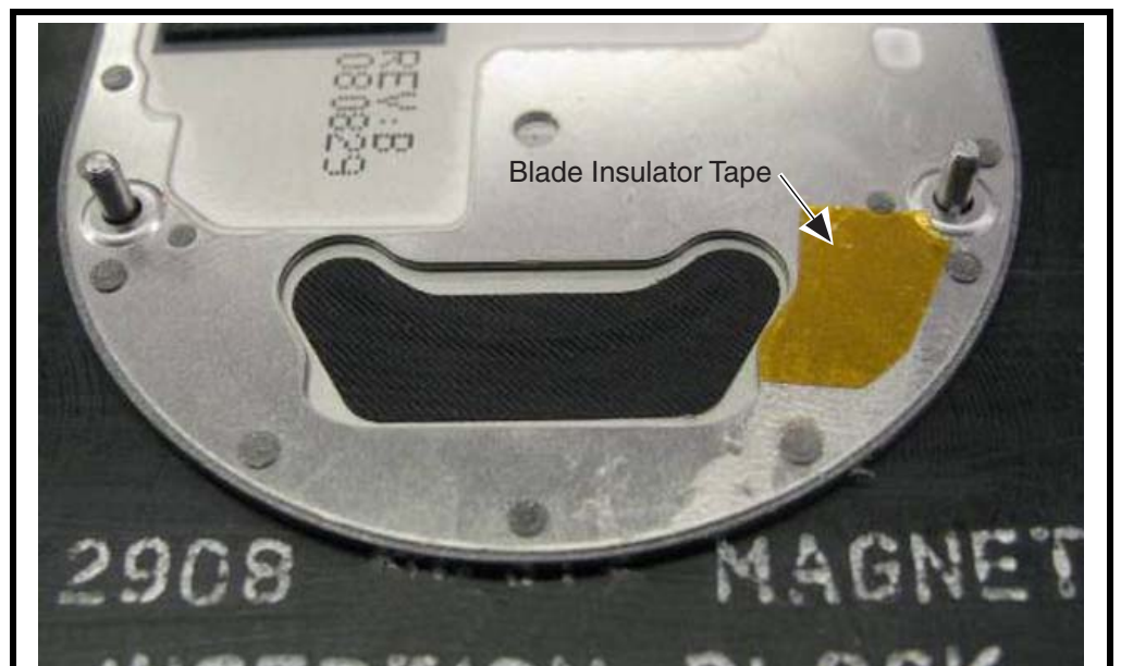
Figure 42. Attaching the Blade Insulator Tape
