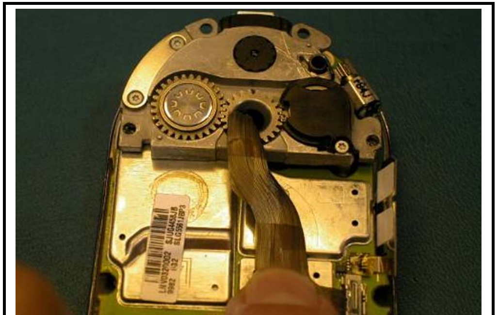
Figure 96. Adhering the Coax Assembly to Memory Shield
