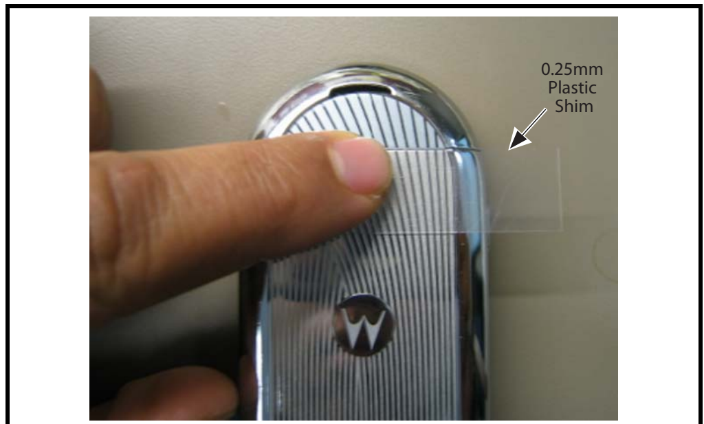
Figure 115. Testing the 0.25 PSCD Requirement
