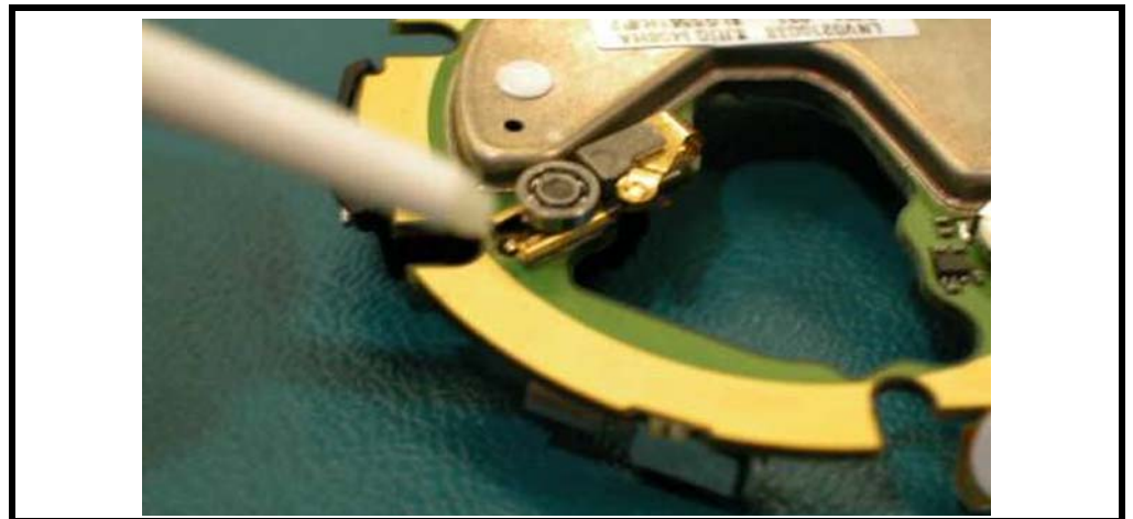
Figure 75. Installing the Detent Bearing-Slider Assembly
