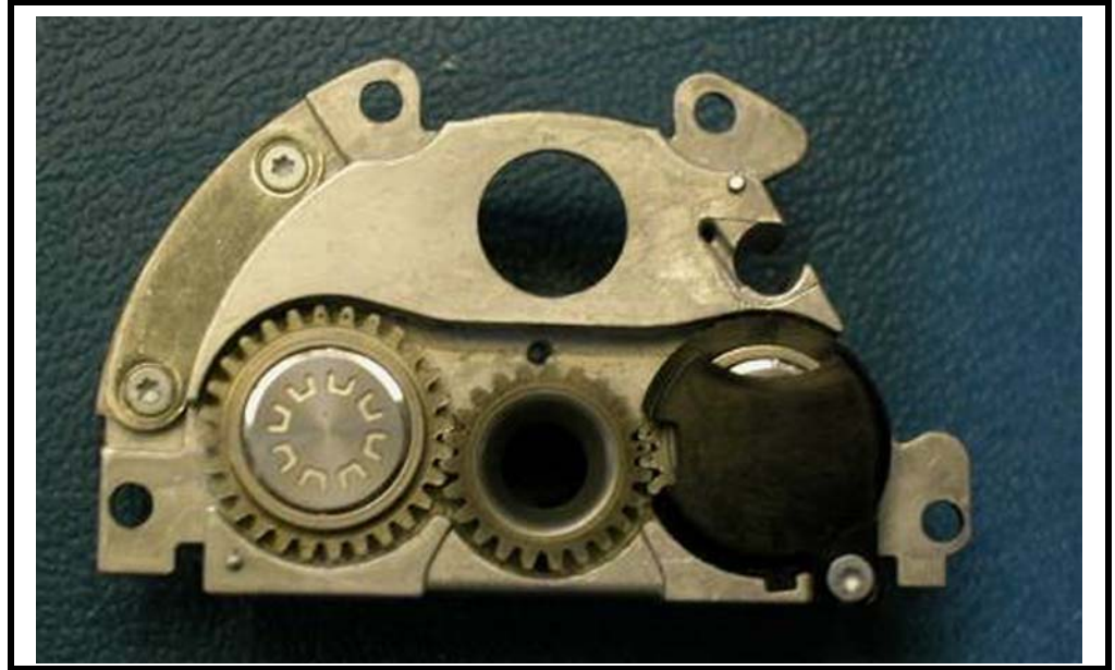
Figure 83. Verifying the Hinge Timing Lock
