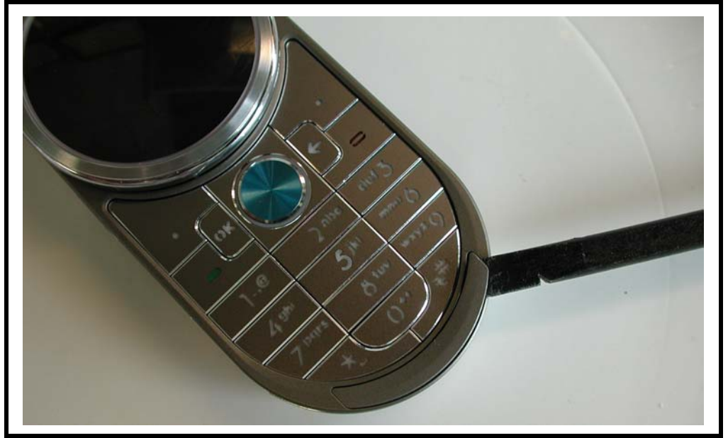
Figure 7. Removing the Escutcheon
