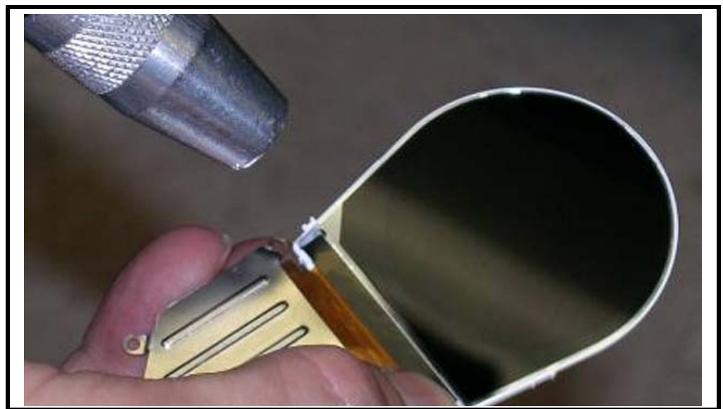
Figure 33. Cleaning the Display Module
