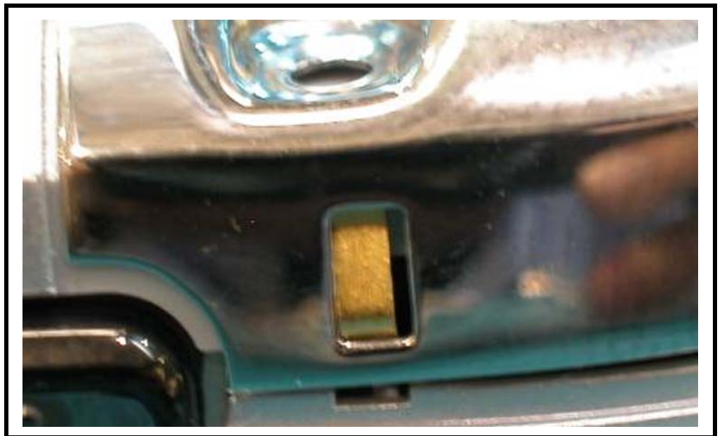
Figure 111. Checking the Grounding Contacts on the Rear Housing
