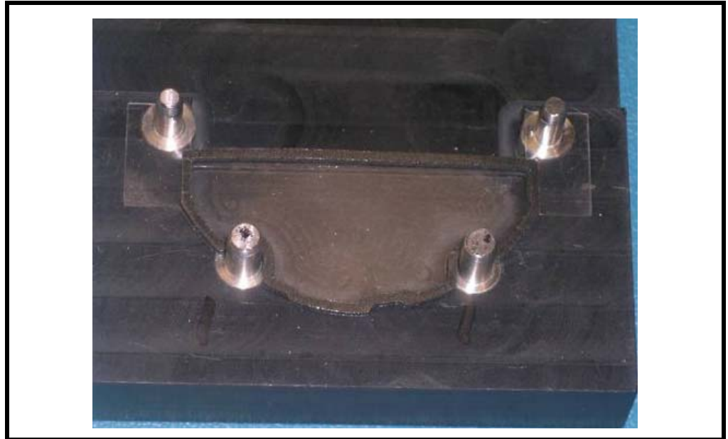
Figure 66. Placing the Acoustic Seal and Top Liner on the Alignment Fixture
