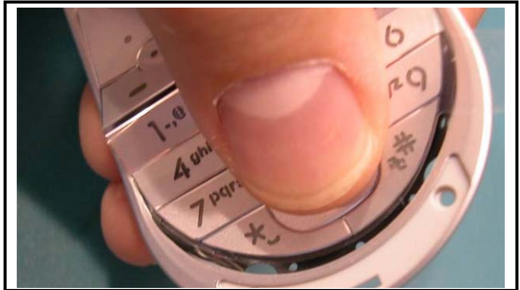
Figure 58. Aligning the Keypad to the Front Housing
