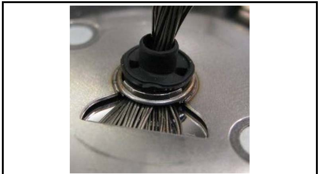
Figure 79. Inserting the Grommet into the Coupler Recesses
