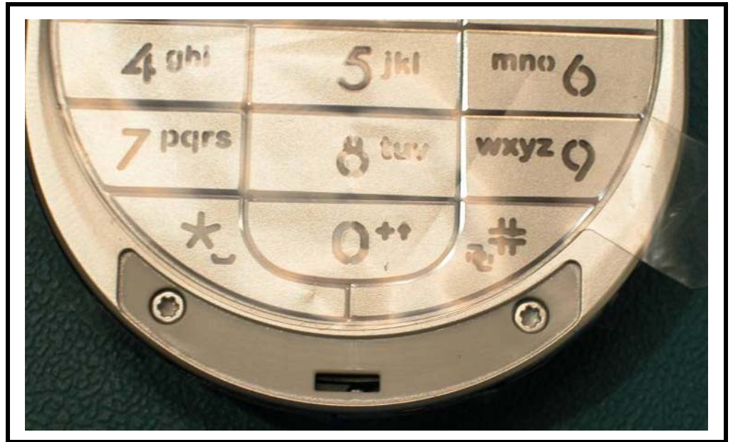
Figure 113. Driving the Antenna Cap Screws
