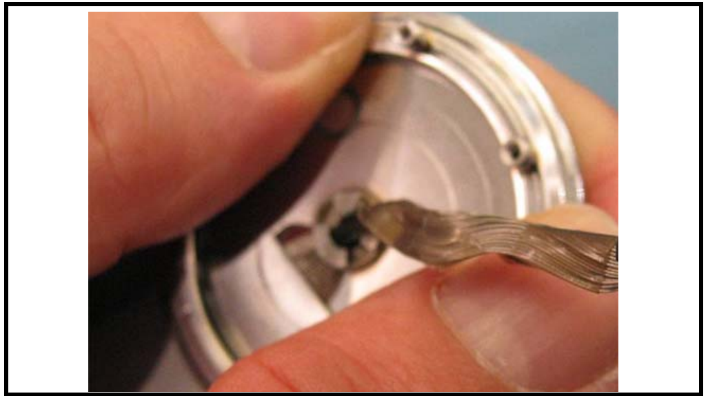
Figure 53. Aligning the Blade Plate Assembly
