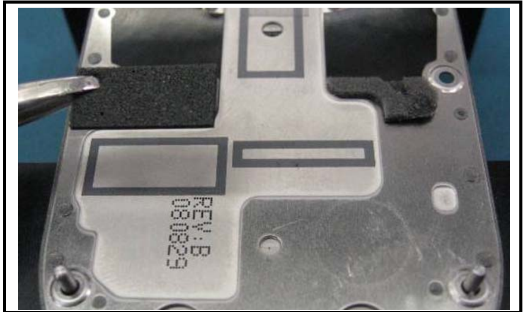
Figure 41. Attaching the Display Backer Pad
