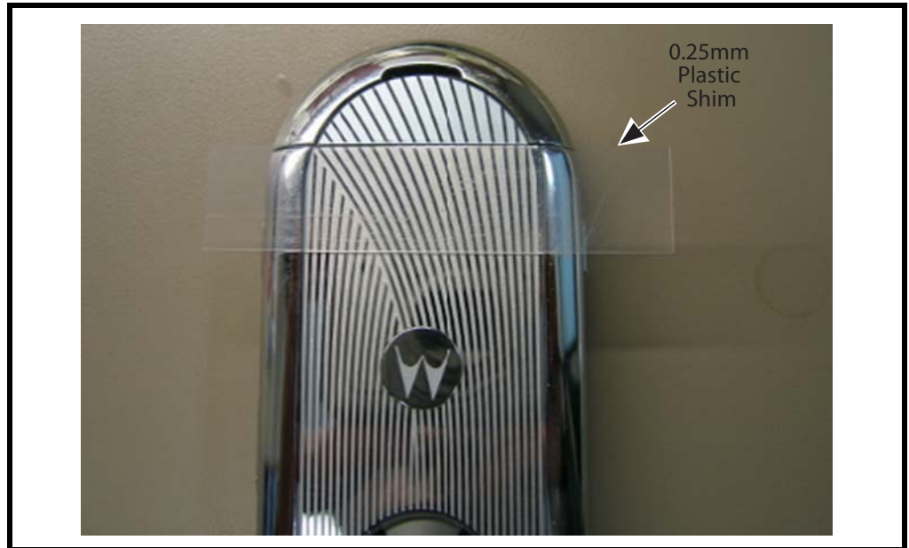
Figure 114. Placing the Plastic Shim
