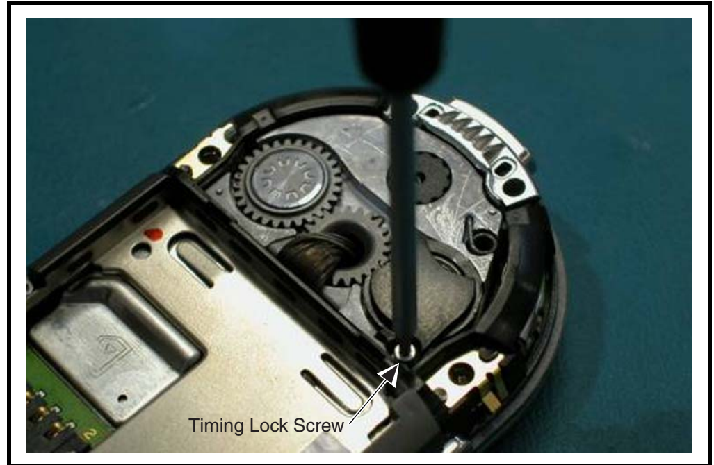
Figure 106. Removing the Timing Lock Screw
