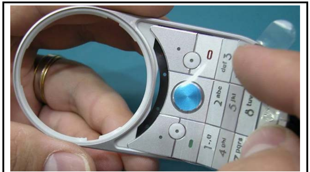
Figure 57. Bending the Keypad While Inserting it onto the Front Housing
