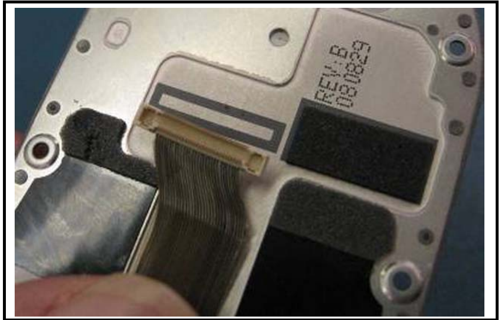
Figure 47. Aligning the Coax Connector
