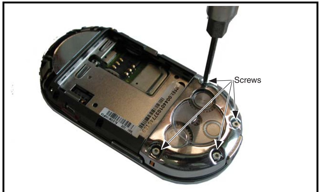
Figure 9. Removing the 4 Top Cap Screws
