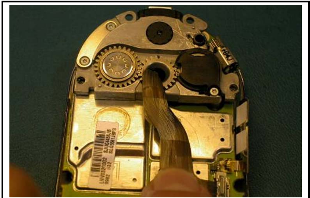
Figure 92. Adhering the Coax Assembly to Memory Shield
