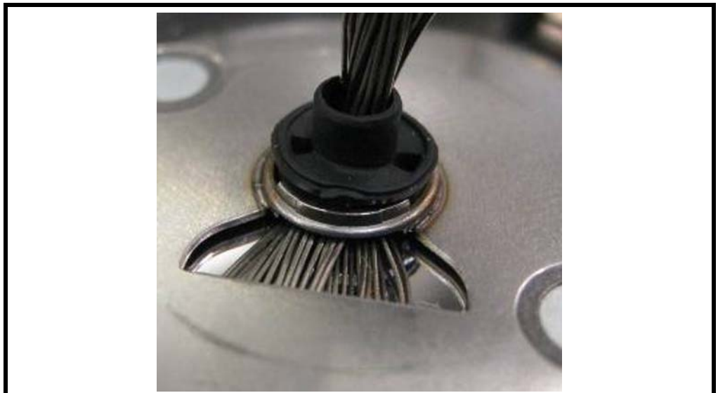
Figure 79. Inserting the Grommet into the Coupler Recesses
