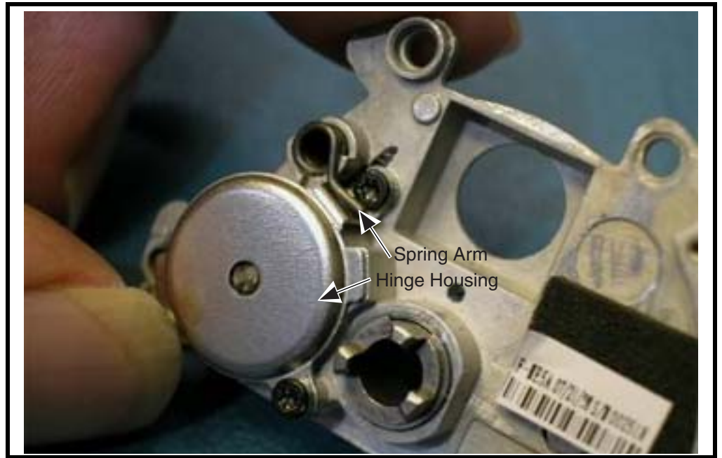
Figure 86. Hinge Module Assembly
