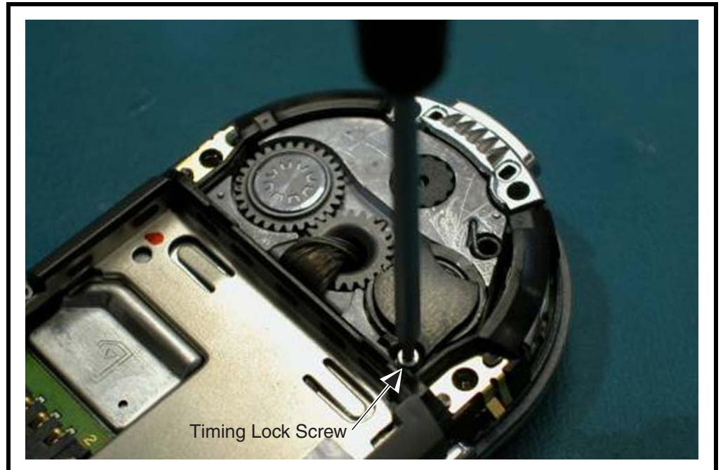
Figure 102. Removing the Timing Lock Screw
