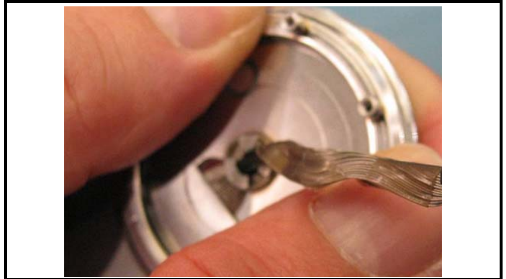
Figure 53. Aligning the Blade Plate Assembly
