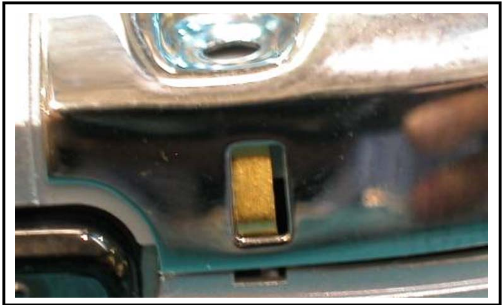
Figure 107. Checking the Grounding Contacts on the Rear Housing
