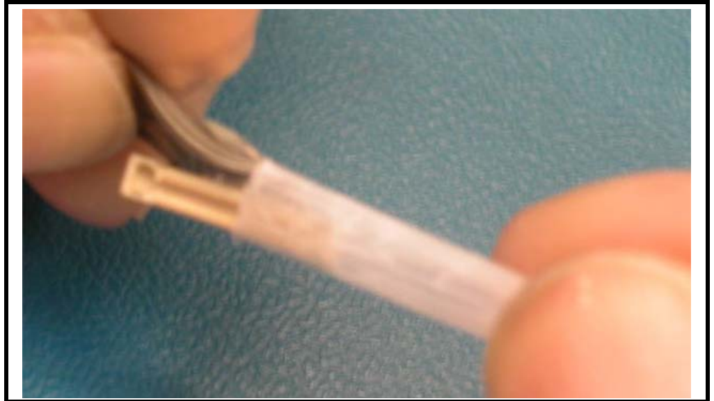
Figure 21. Protecting the Coaxial Connector Protective Cap
