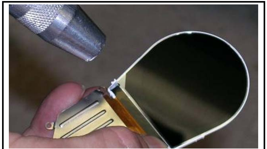
Figure 33. Cleaning the Display Module
