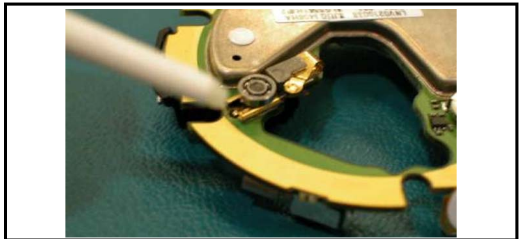
Figure 75. Installing the Detent Bearing-Slider Assembly
