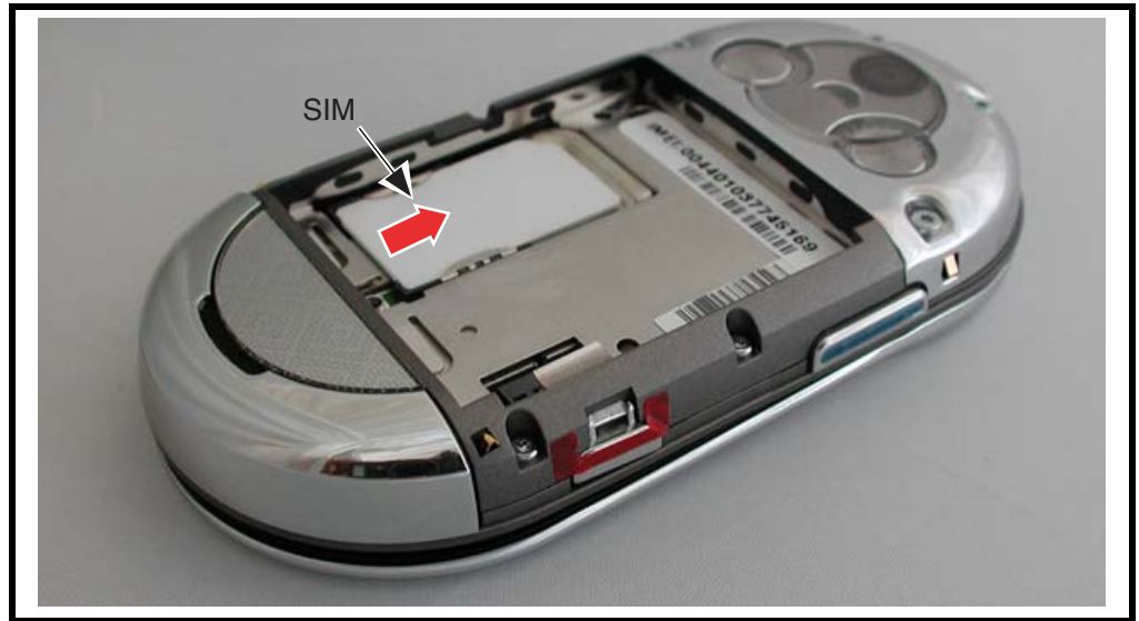
Figure 6. Removing the SIM
