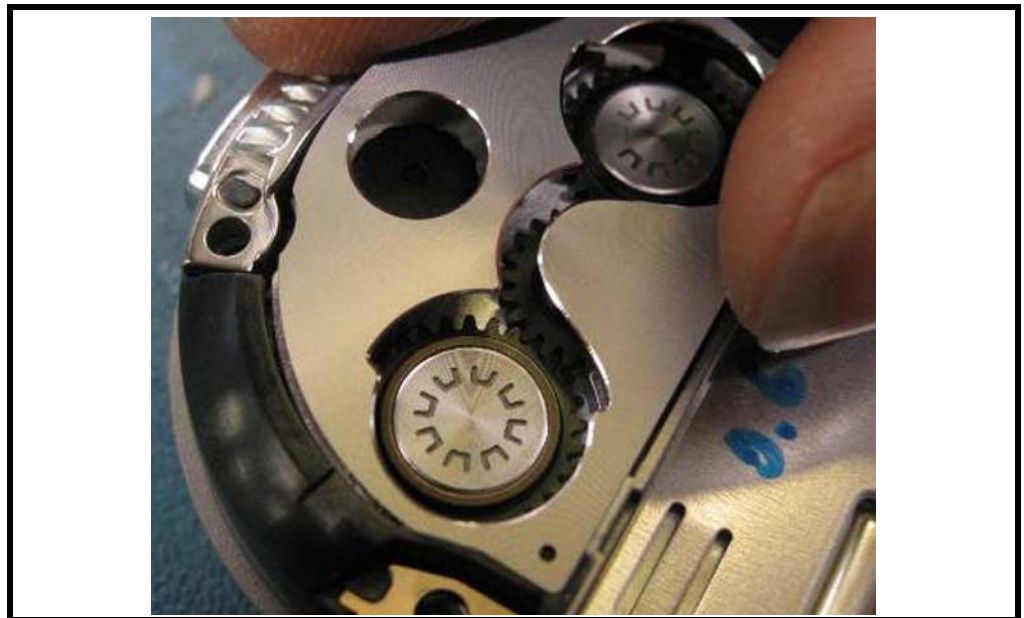
Figure 104. Attaching the Hinge Bezel
