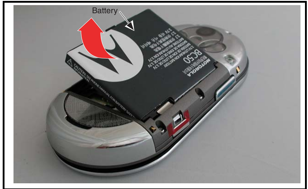
Figure 5. Removing the Battery
