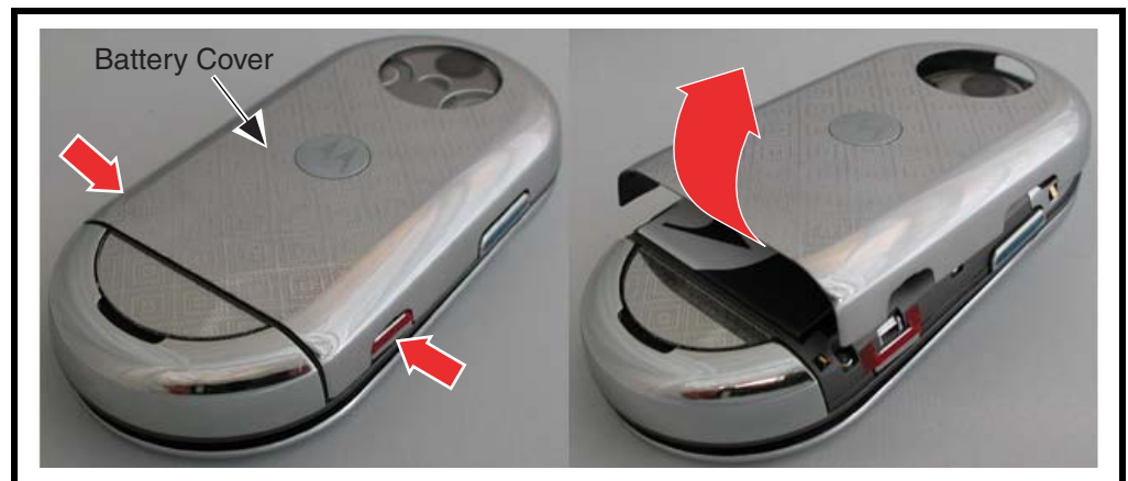
Figure 4. Removing the Battery Cover
