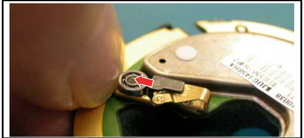
Figure 76. Pushing the Detent Bearing-Slider Assembly
