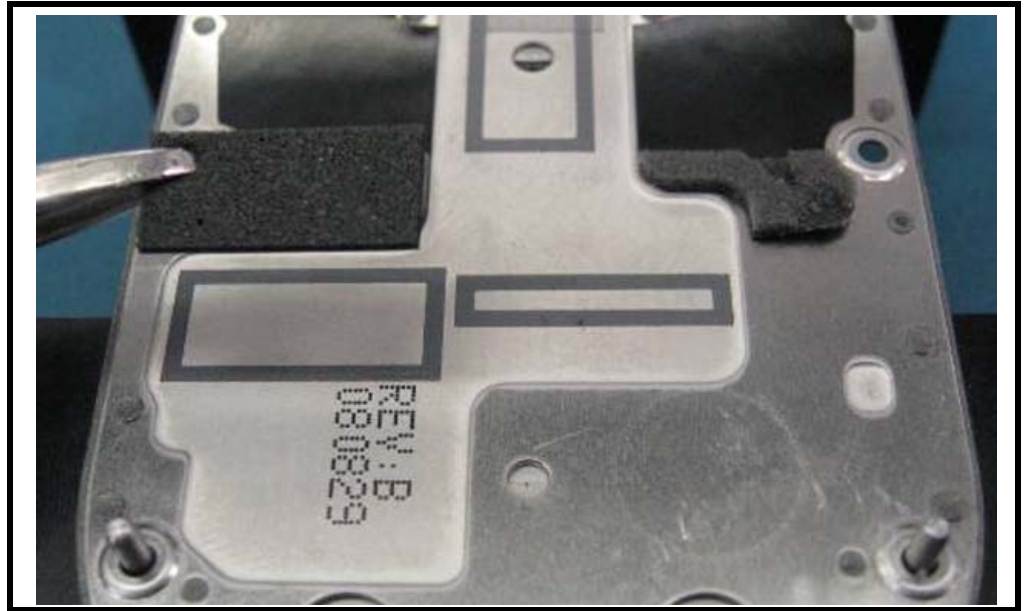
Figure 41. Attaching the Display Backer Pad
