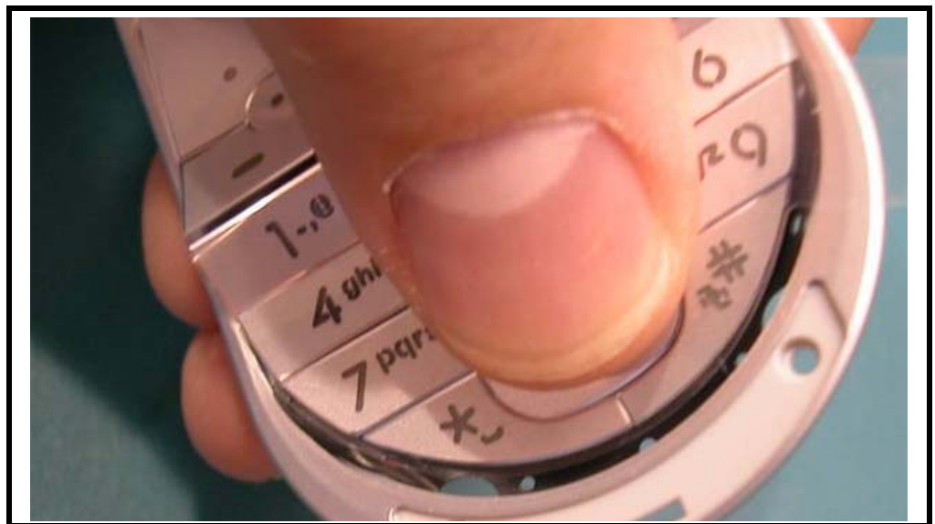
Figure 58. Aligning the Keypad to the Front Housing
