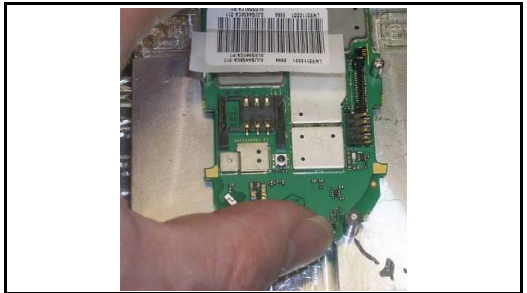
Figure 61. Inserting the PCB onto the Dome Array Alignment Fixture
