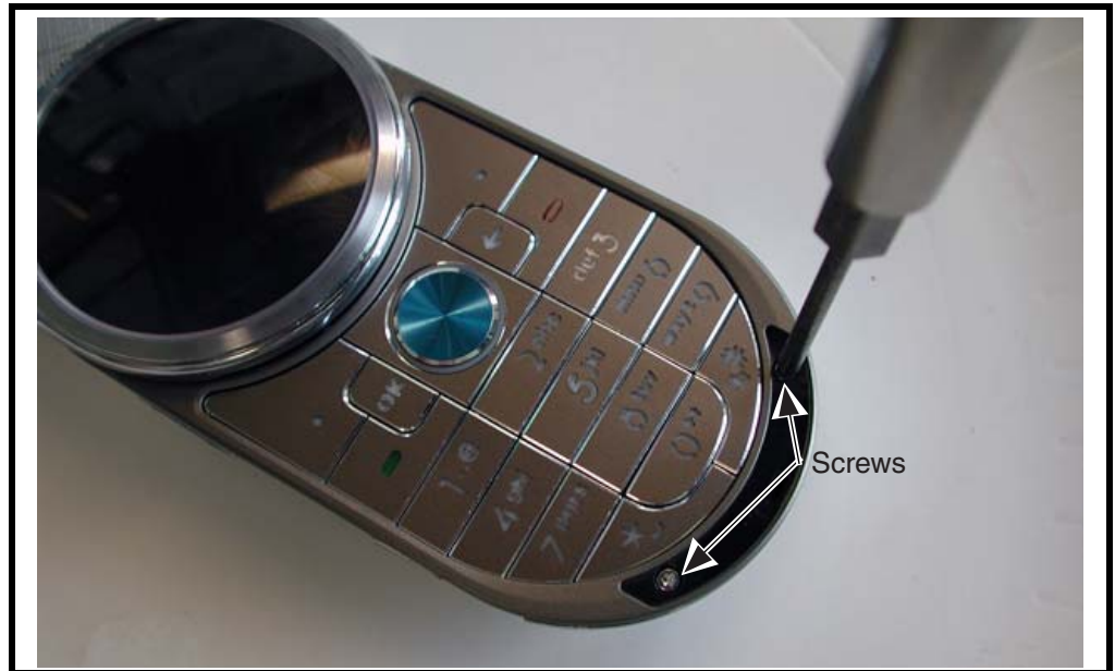
Figure 8. Removing the Transceiver Housing Screws
