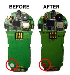
WATER DETECT LABEL WHITE - NORMAL BEFORE LIQUID CONTAMINATION WATER DETECT LABEL TURNS RED AFTER LIQUID CONATAMINATION
