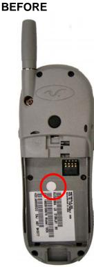
WATER DETECT LABEL WHITE - NORMAL BEFORE LIQUID CONTAMINATION
