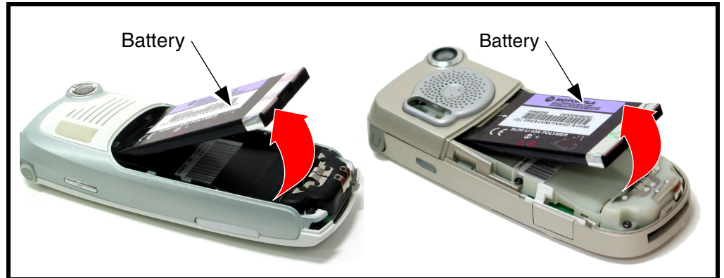
Figure 4. Removing and Replacing the Battery
