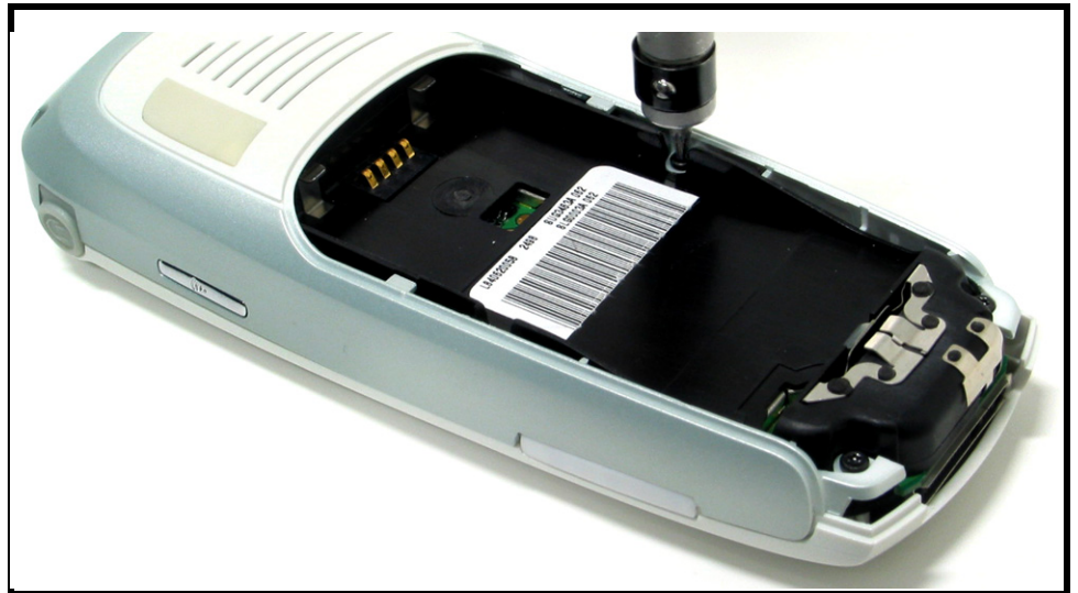
Figure 6. Rear Housing Screws Removal
