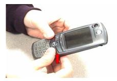
Classification: Motorola Internal Information Strictly released for Motorola Authorized Service Center Use only. 3. Secure the unit with your left hand by firmly pressing down on the keypad and holding the rear of the unit. With your right thumb, expand the right side of the housing by pulling your thumb in the direction of the red arrow. Once the screw boss is clear, lift the right hand side of the housing using your thumb and index finger around the keypad.
