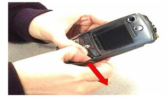
4. Once the right side of the housing is apart, use your right hand to secure the unit. Flex the left side of the housing using your left thumb as show by the red arrow. Once the screw boss is clear of the keypad, lift housing off the unit.
