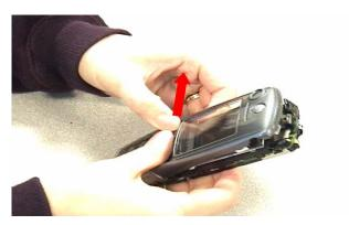
5. Once the screw boss is clear of the keypad, lift the housing off the unit as show below.
