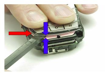
8. Carefully continue to insert the plastic disassembly tool to break the adhesive bond between the keypad and the EL backlighting as shown in the following pictures. Do not tear off the keypad at anytime. Continue to use the plastic disassembly tool to lift the keypad off.
