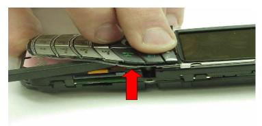
10. Continue to insert plastic disassembly tool until keypad is no longer adhered to the EL back lighting.
