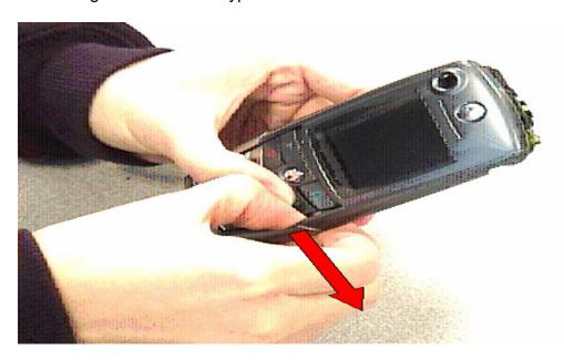
4. Once the right side of the housing is apart, use your right hand to secure the unit. Flex the left side of the housing using your left thumb as show by the red arrow. Once the screw boss is clear of the keypad, lift housing off the unit.
