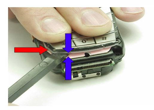
9. Carefully continue to insert the plastic disassembly tool to break the adhesive bond between the keypad and the EL backlighting as shown in the following pictures. Do not tear off the keypad at anytime. Continue to use the plastic disassembly tool to lift the keypad off.
