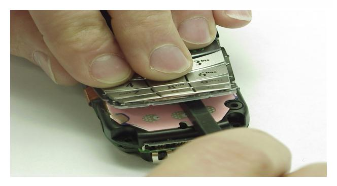
10. As you continue to insert the plastic disassembly tool down the right side of the phone as shown below, be careful not to damage the second EL bond. The red arrow shows the location of the EL bond.
