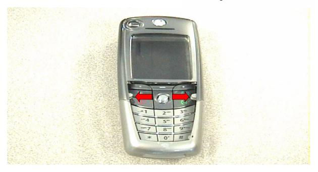
2. The First step is to flex the right hand side of the housing. The red area below shows where the screw boss is that needs to clear the keypad during disassembly.
