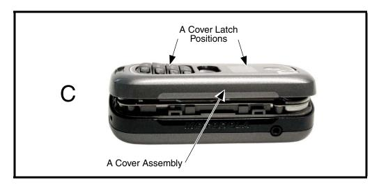
Figure 15. Removing the A Cover Assembly Part 2
