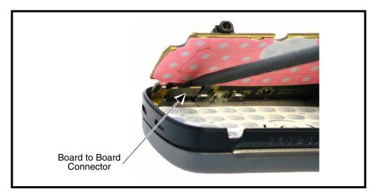
Figure 10. Disconnecting the Board to Board Connector
