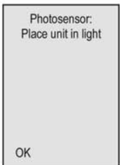
Expose keypad to light source. Press left Option key when ready
