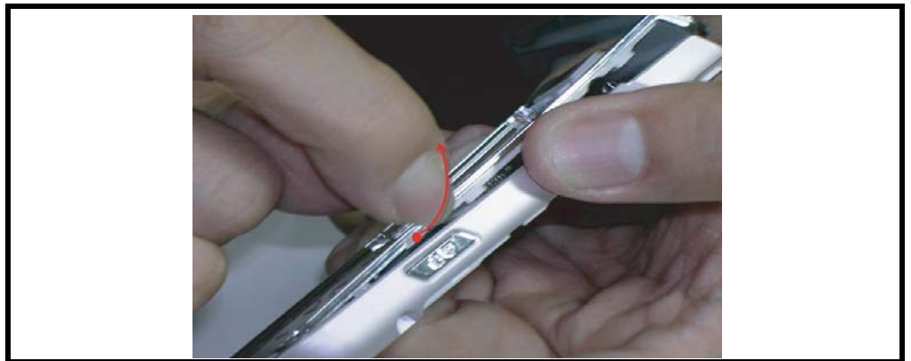
Figure 35. Removing Case C and Case D
