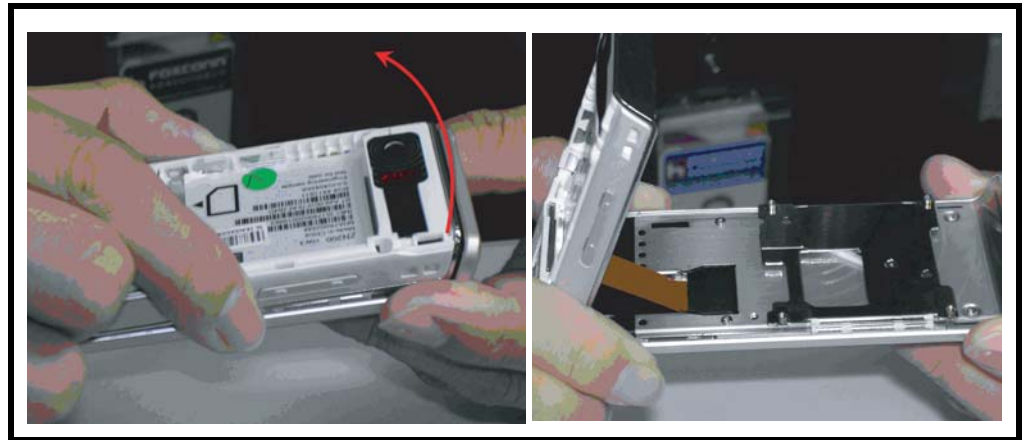
Figure 10. Separate the Lower module from Upper module.
