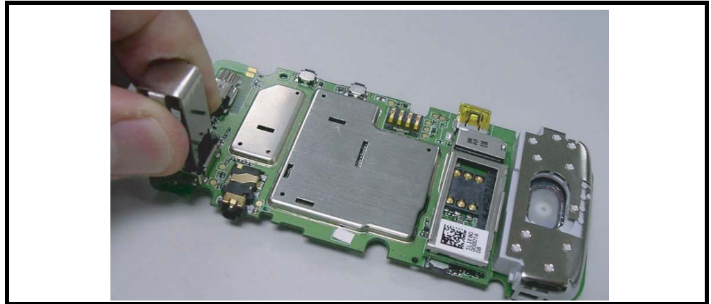
Figure 46. Removing the Antenna Carrier
