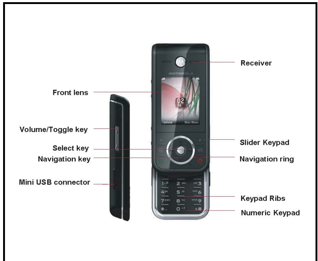
Figure 1. ZN200 Telephone Controls Locations
