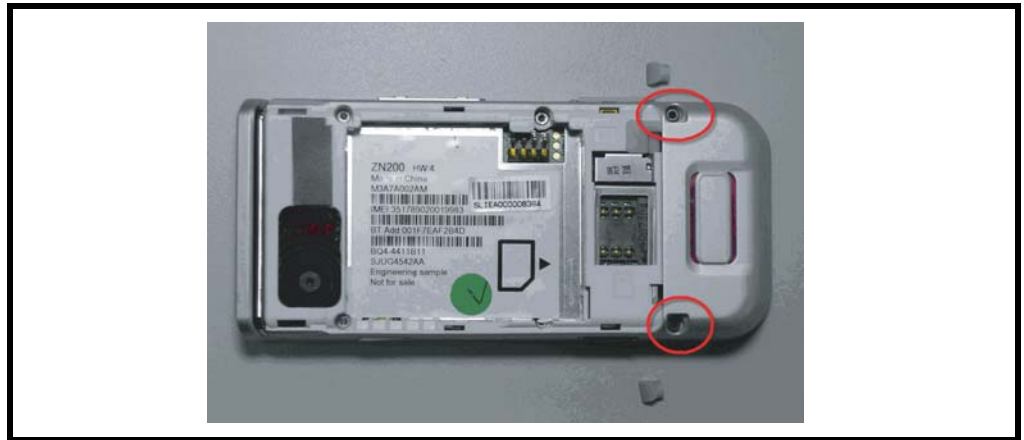
Figure 8. Removing the screw covers
