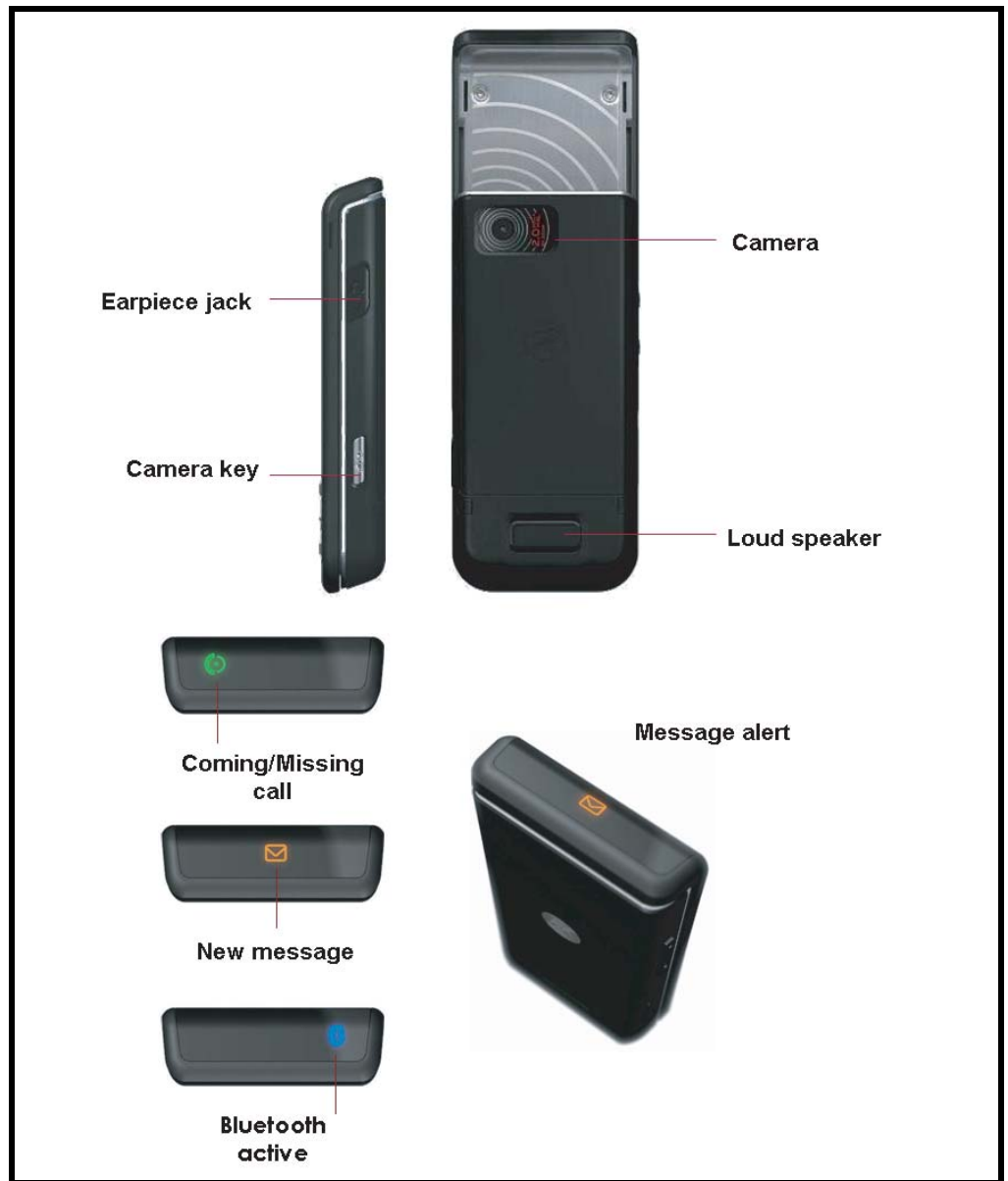
Figure 2. ZN200 Telephone Controls Locations
