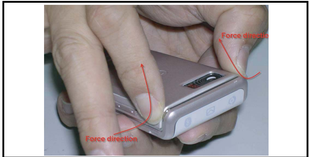
Figure 6. Removing the Battery Door
