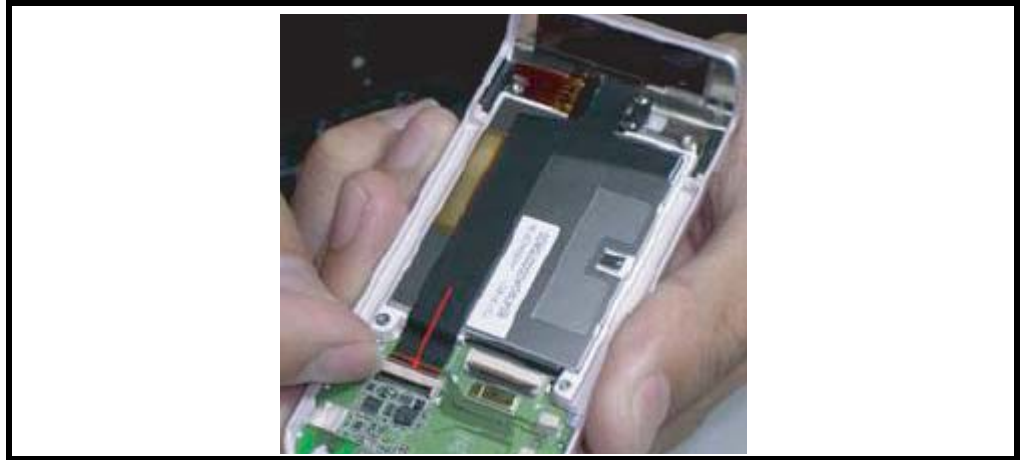
Figure 22. Assembly the LCM FPC
