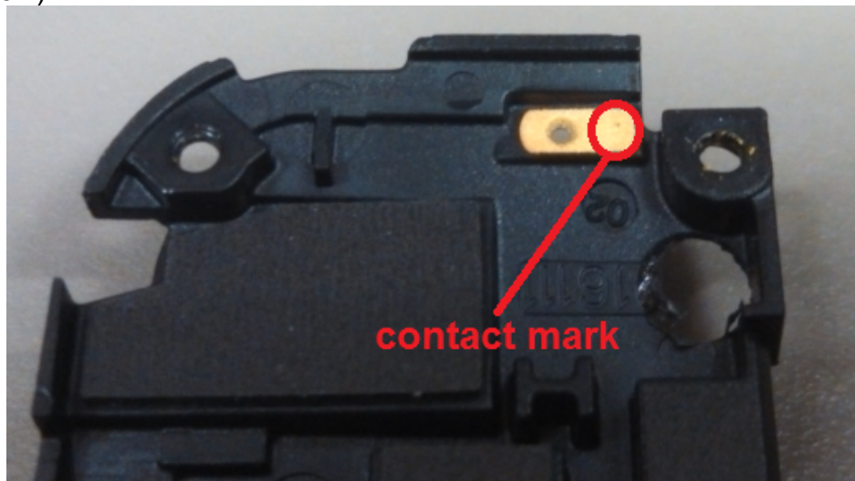
Figure: Contact Mark in Antenna 5, near Front Facing Imager side
