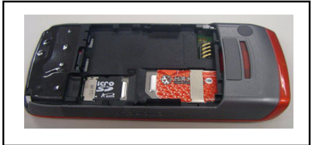
Figure 7. Removing the T-flash card
