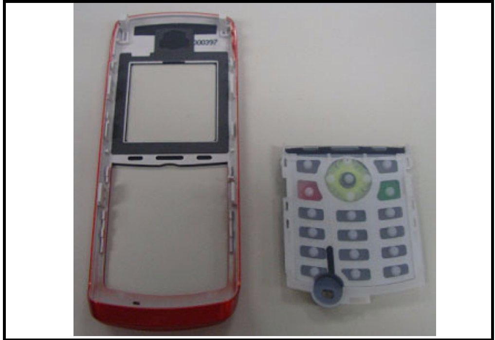
Figure 13. Removing the rubber keypad
