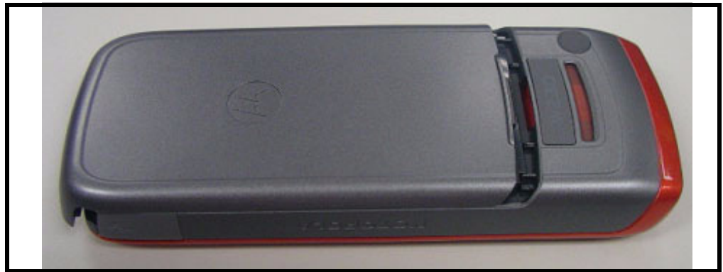
Figure 5. Removing the battery cover
