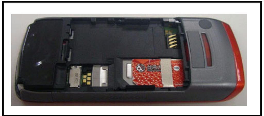
Figure 8. Removing the SIM card
