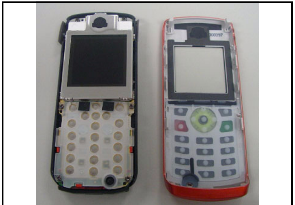
Figure 12. Removing the front housing
