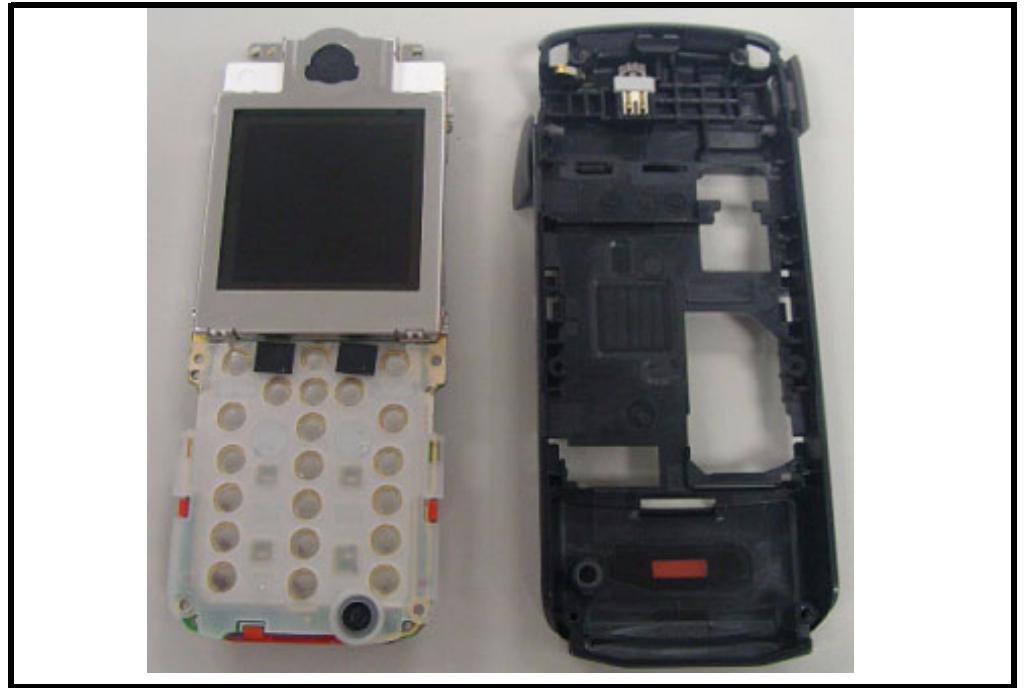
Figure 15. Disengaging the side hooks
