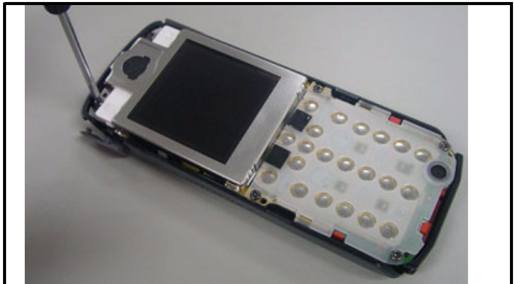
Figure 14. Removing the six T5 screws
