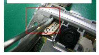
Use the disassemble hook to disassemble the hinge KB
