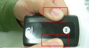
To press the both side of the display upper case and lower case to assemble the both side hooks
