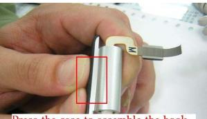
Press the case to assemble the hook
