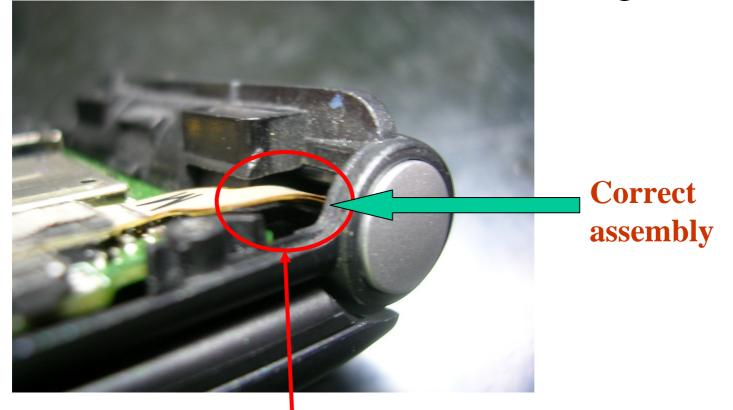
The Hinge FPC pass through the slot of Hinge\_Kb.
