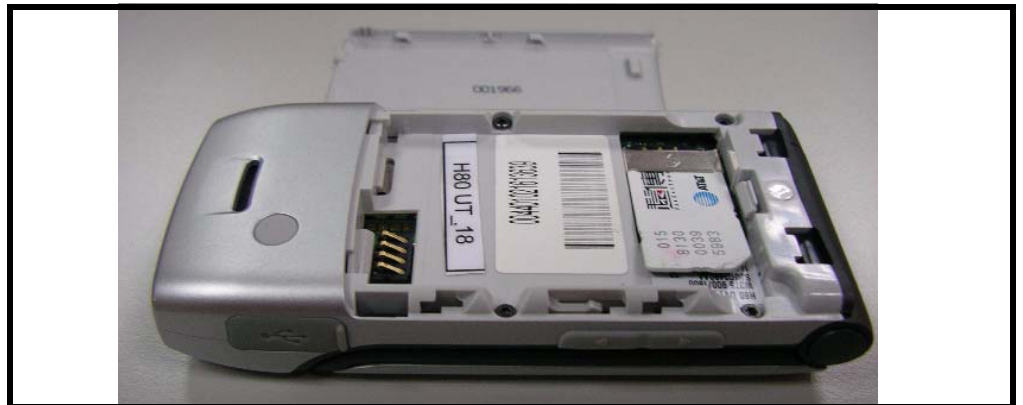
Figure 7. Removing the SIM Card
