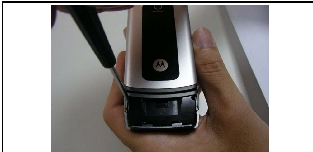
Figure 9. Removing the screws
