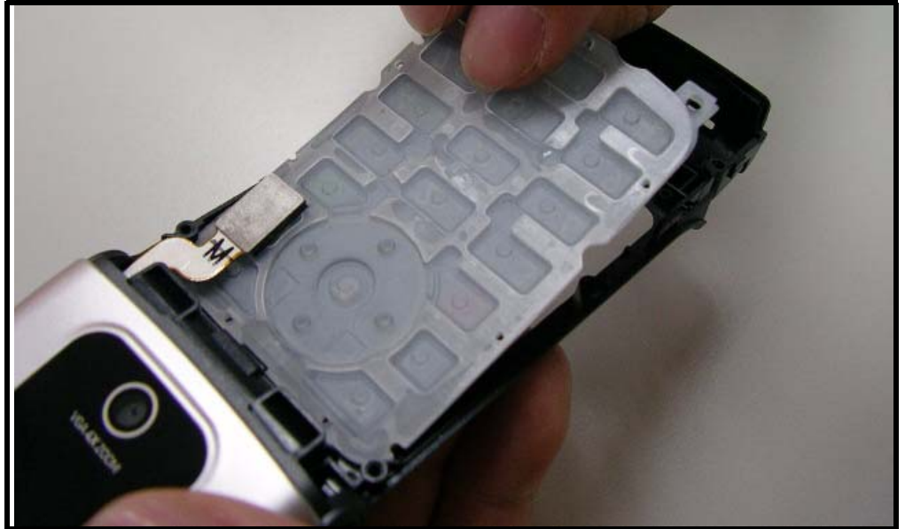
Figure 25. Removing the keypad
