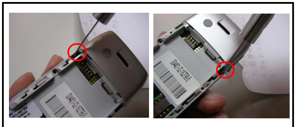
Figure 12. Disengaging the latches
