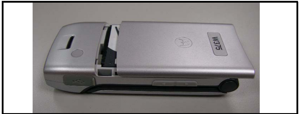
Figure 5. Opening the battery cover
