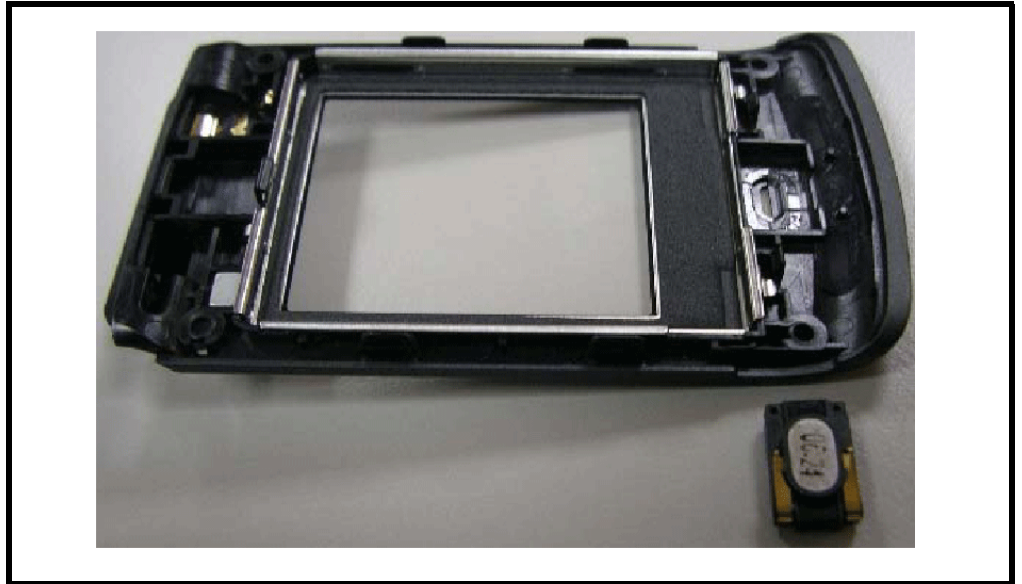
Figure 41. Removing the receiver
