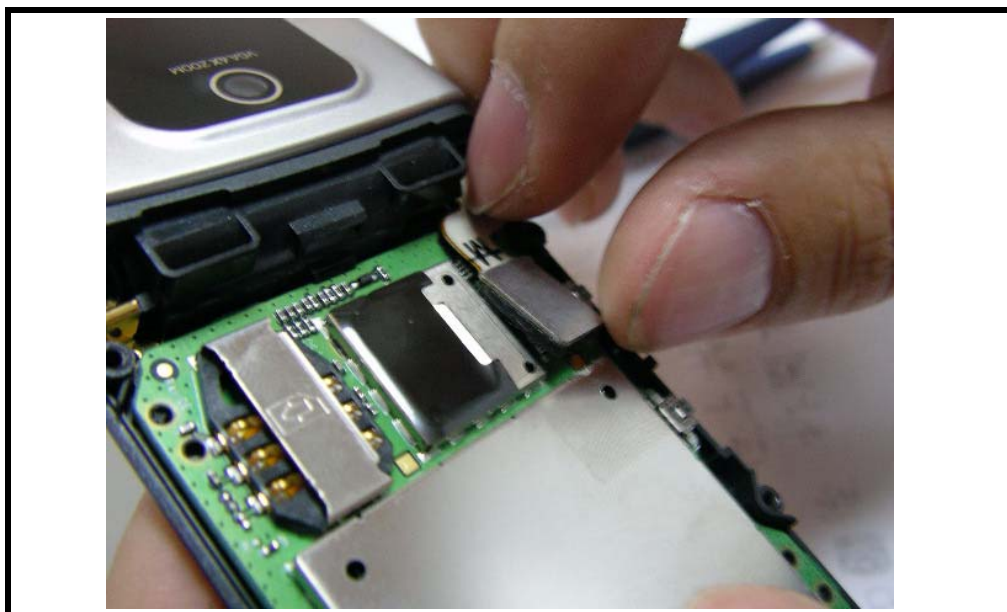
Figure 20. Prying off the FPC connector
