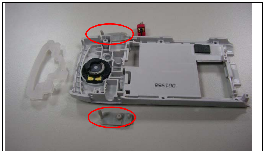
Figure 16. Removing the rubber pad
