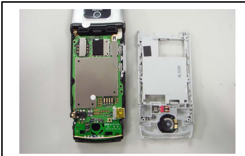
Figure 13. Separating the back housing
