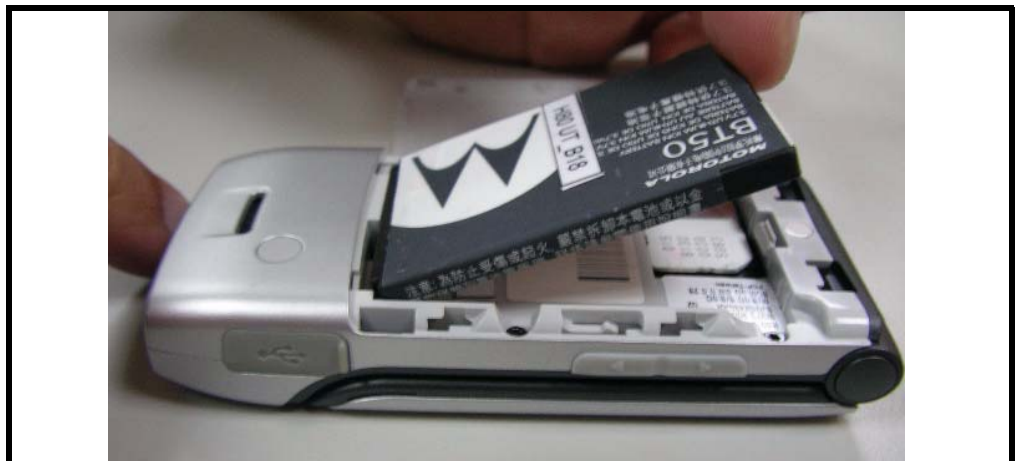
Figure 6. Removing the battery
