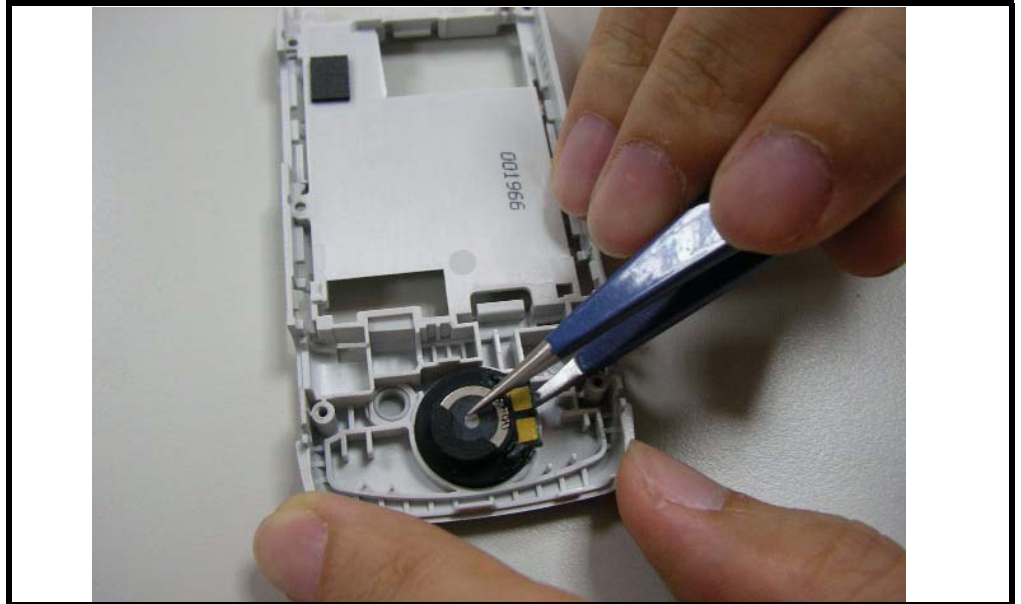
Figure 17. Removing the speaker chip
