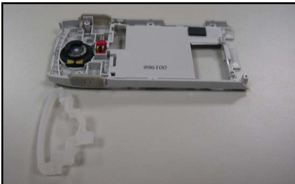
Figure 14. Removing the Spk-gasket
