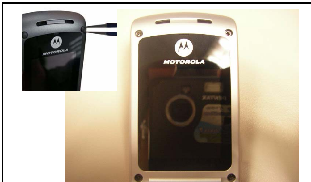
Figure 27. Remove four rubber cover
