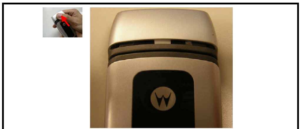
Figure 8. Removing the cap
