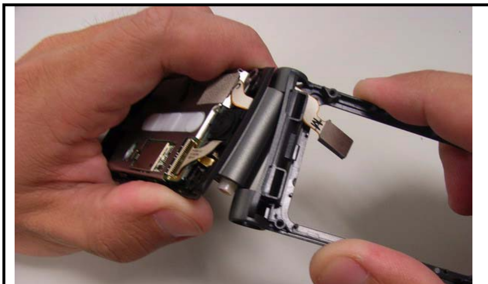
Figure 34. Disconnecting the top clamshell
