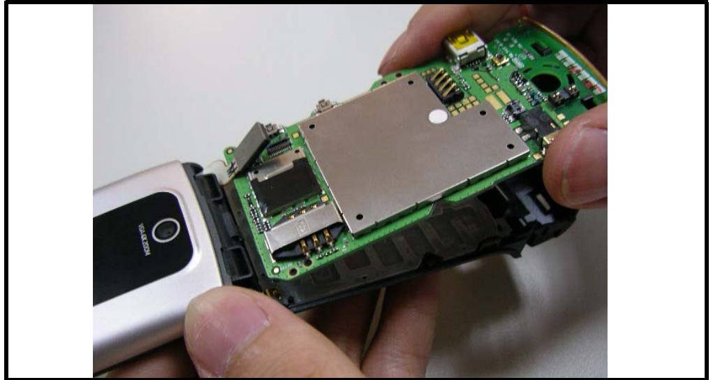
Figure 21. Remove the main board
