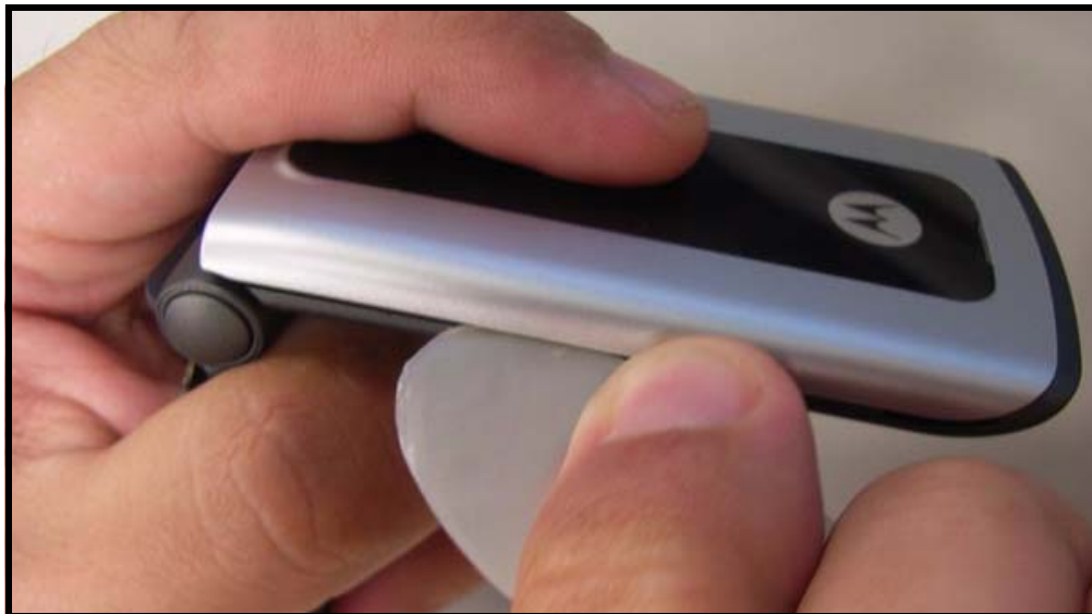
Figure 29. Disconnecting the two halves
