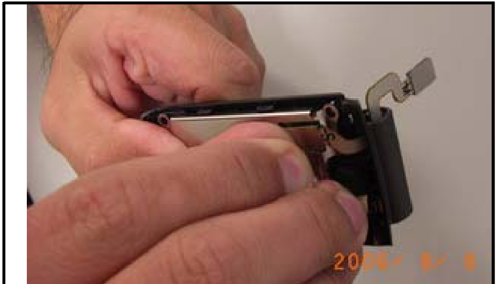
Figure 36. Prying off the FPC connector
