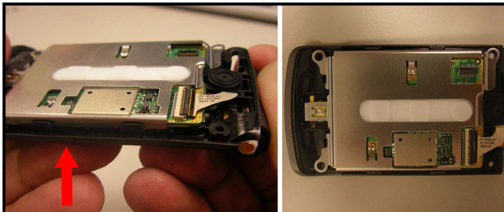
Figure 37. Disengaging the latches
