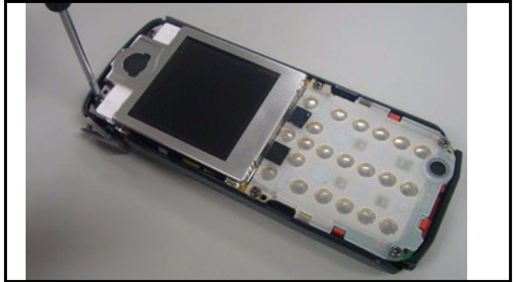
Figure 11. Removing the six T5 screws
