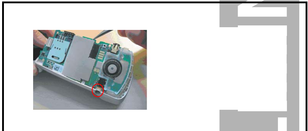
Figure 16. Replacing PCBA to lower housing cover
