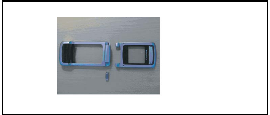
Figure 44. Separating Case-B, Case-C, and the hinge
