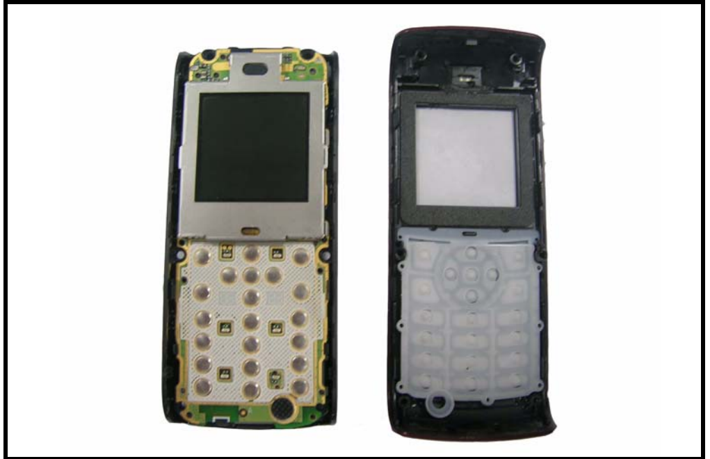
Figure 11. Removing the front housing
