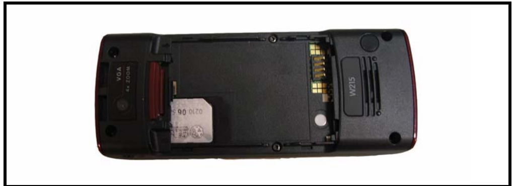
Figure 7. Removing the SIM card
