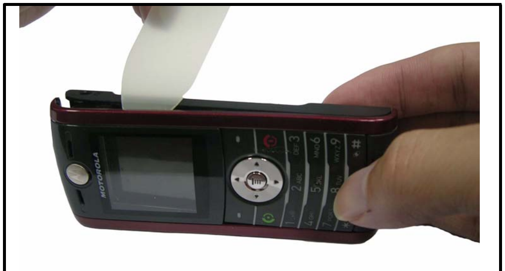
Figure 10. Prying the case apart along the seam
