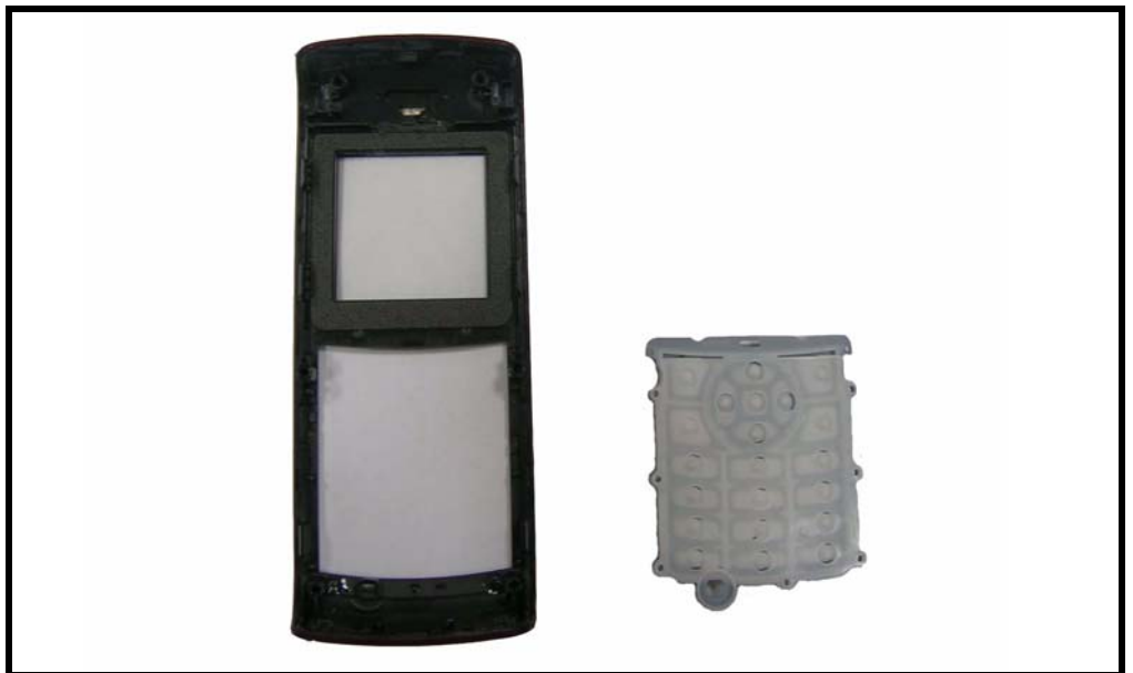
Figure 12. Removing the rubber keypad
