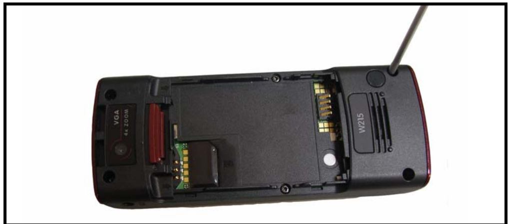
Figure 8. Removing the six T5 screws
