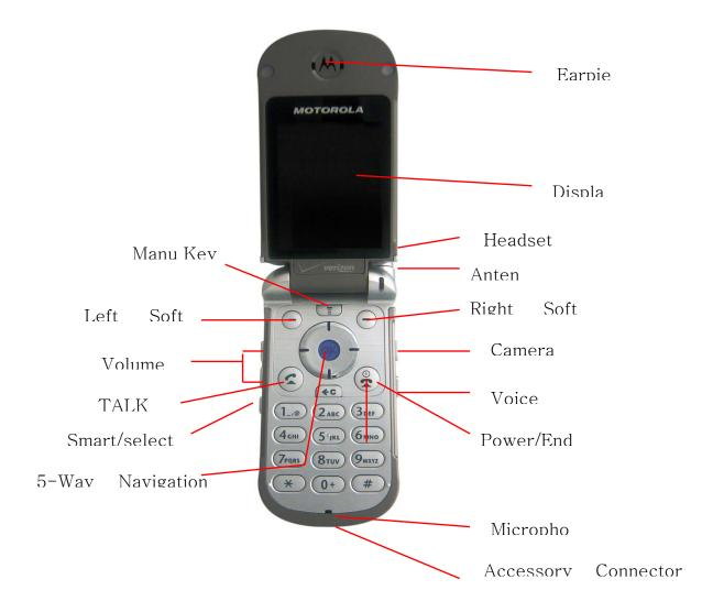
The flip assembly includes the entire hinge mechanism and is attached to the main housing by four screws. There is a full display on the inside of the flip assembly and a OLED on the outside of the flip assembly.
