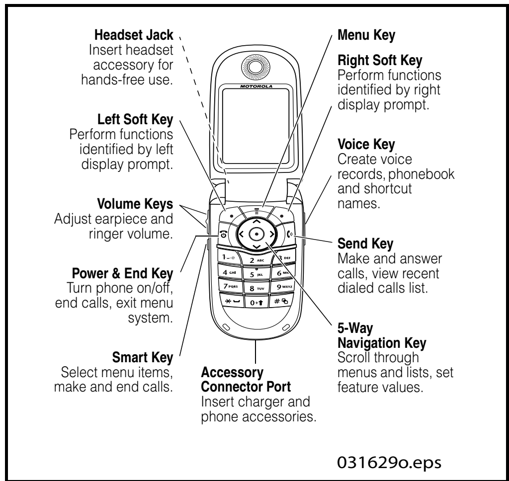
Figure 1. V600 Telephone Controls, indicators, and I/O
