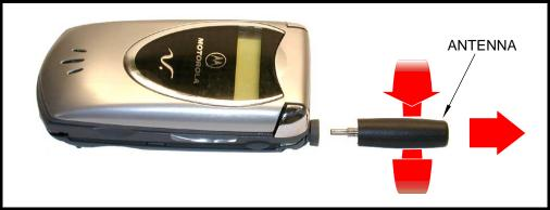
Figure 8. Removing the antenna
