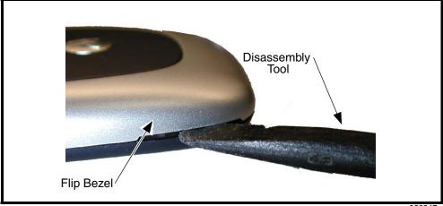
Figure 11. Removing the Flip Bezel
