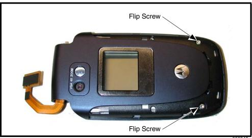
Figure 12. Removing the Flip Assembly Screws
