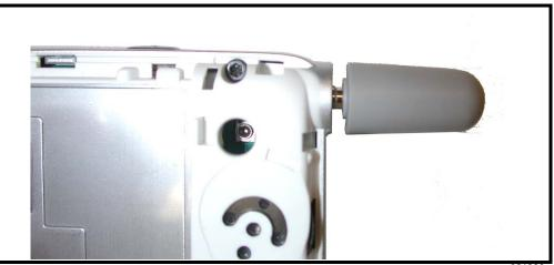
Figure 5. Removing the Antenna
