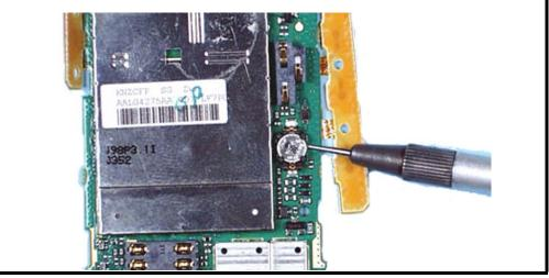
Figure 11. Removing the RTC Battery
