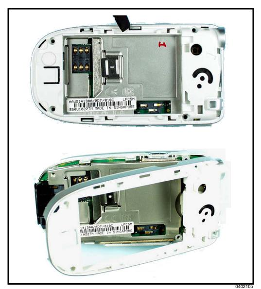
5. Carefully lift the rear housing away from the front housing and flip assembly.
