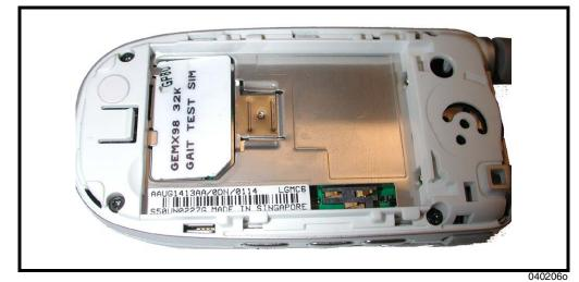
Figure 3. Removing the SIM
