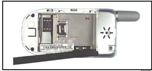
Figure 4. Removing the Polyphonic Speaker Cover
