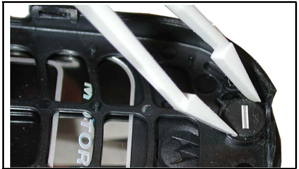
Figure 10. Removing the Microphone and Microphone Grommet
