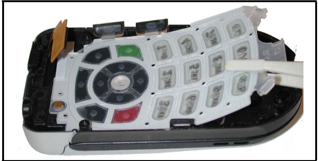
Figure 9. Removing the Keypad
