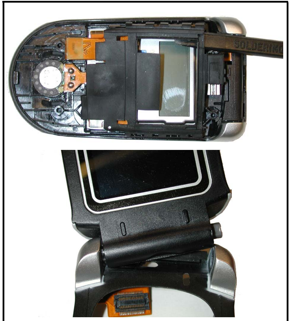
Figure 13. Removing the Flip Assembly
