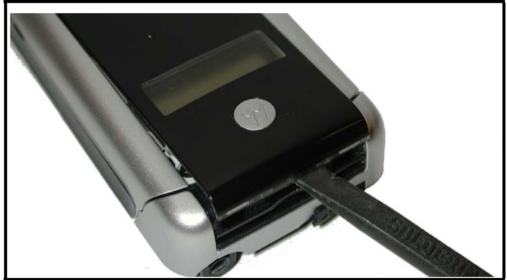
Figure 11. Removing the CLI Lens
