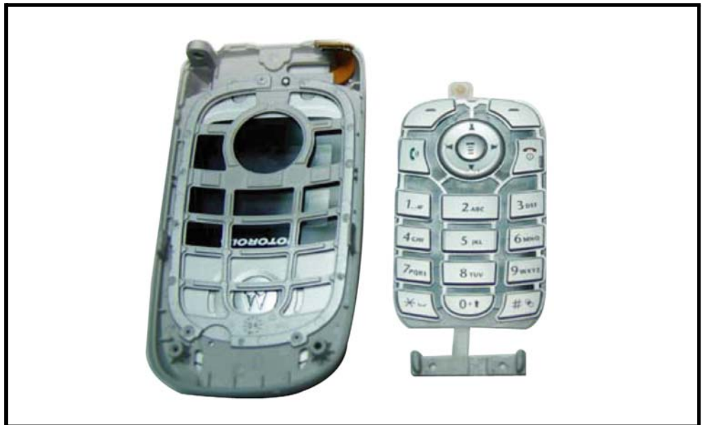
Figure 14. Removing the keypad
