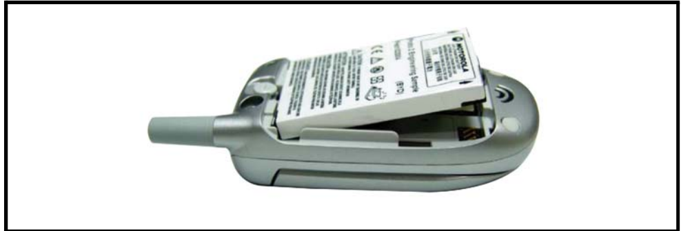
Figure 5. Replacing the battery
