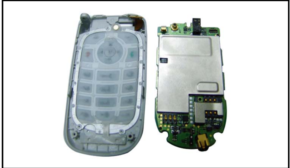
Figure 13. Removing the transceiver board
