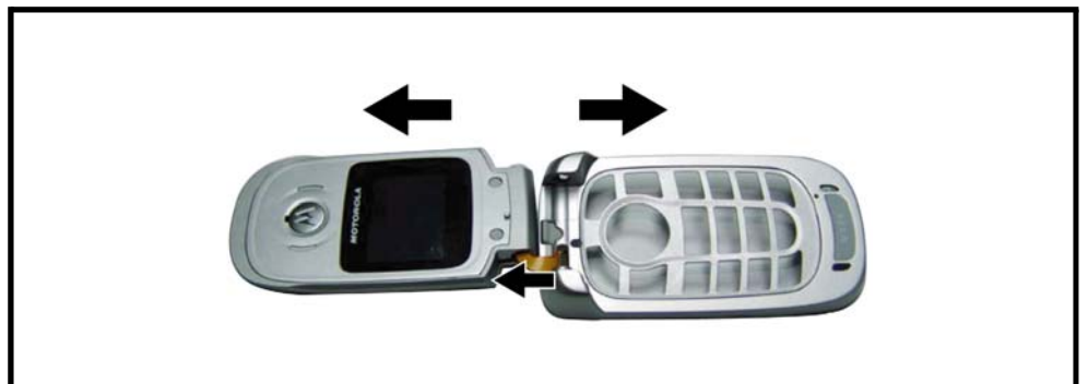
Figure 16. Disconnecting the two halves
