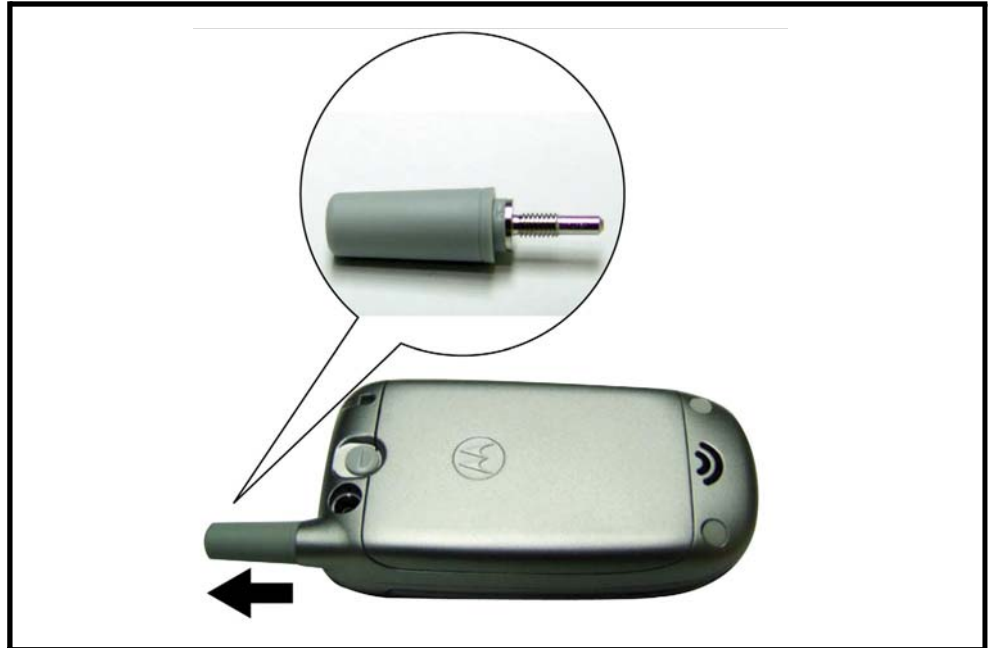
Figure 7. Removing the antenna
