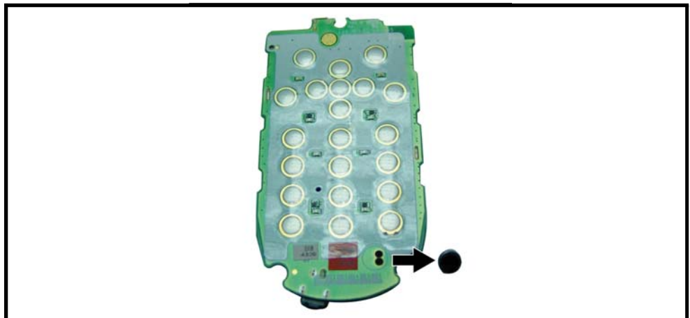
Figure 18. Removing the microphone
