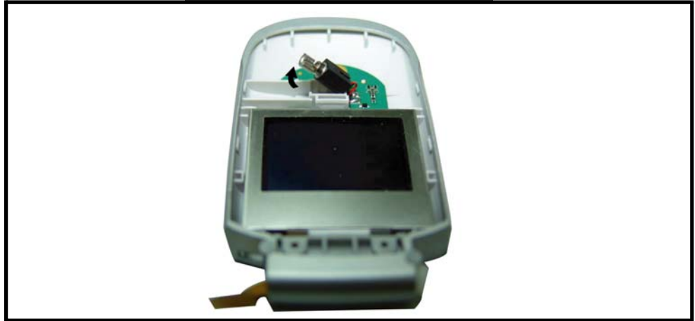
Figure 21. Removing the vibrator
