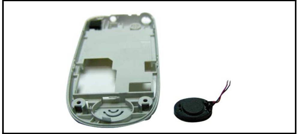
Figure 11. Removing the speaker
