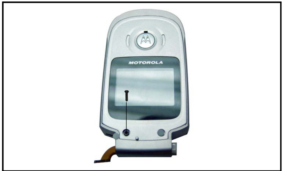
Figure 19. Removing two T5 screws
