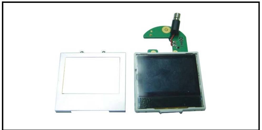
Figure 24. Removing the LCD shielding case
