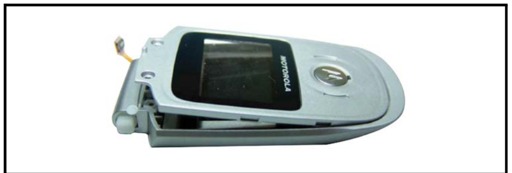
Figure 20. Prying off the front face
