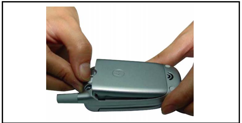
Figure 4. Removing the battery cover
