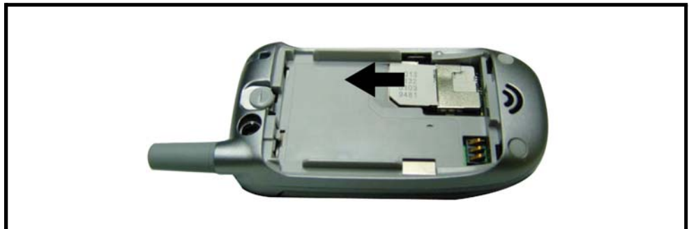
Figure 6. Removing the SIM card
