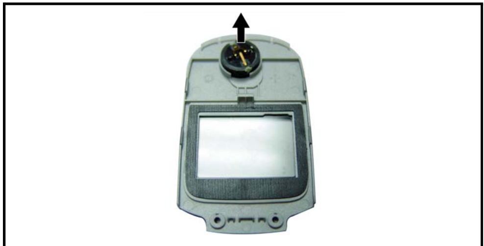
Figure 22. Removing the Receiver
