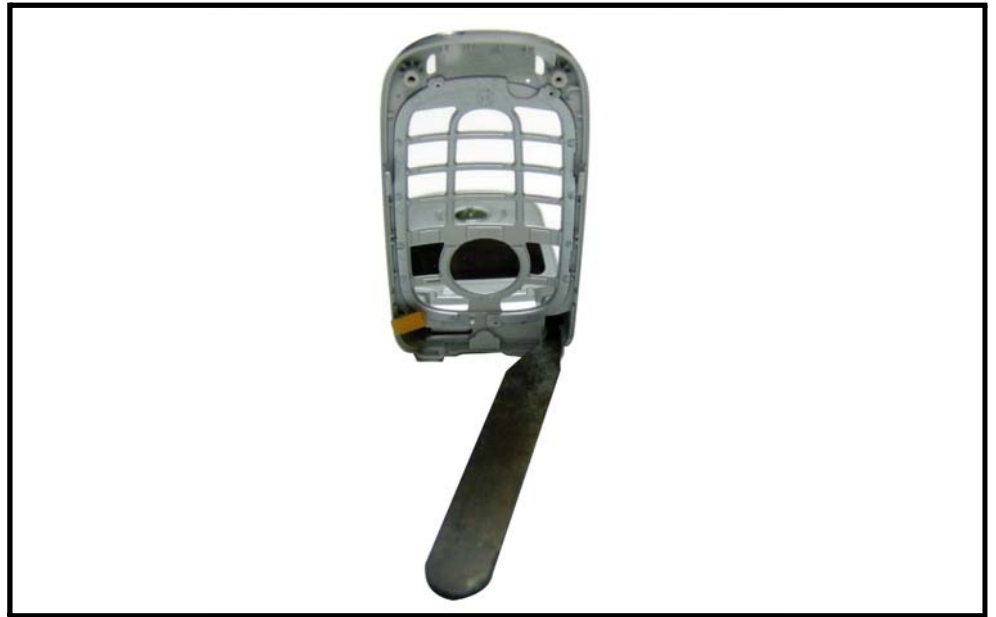
Figure 15. Removing the Flip cover
